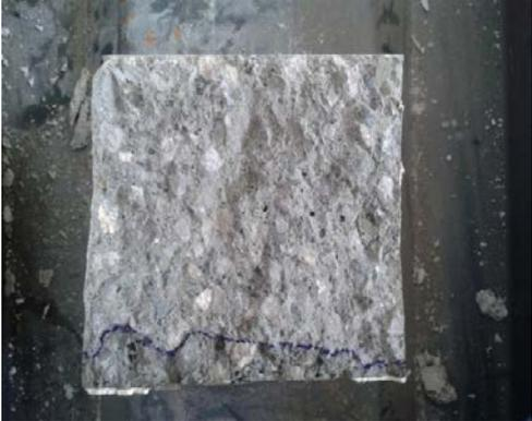
Figure 4: Marked depth of water ingress.
