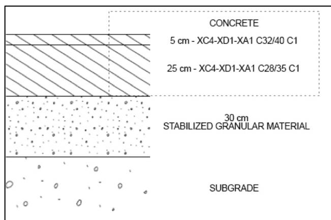
Figure 4: Road cross section
