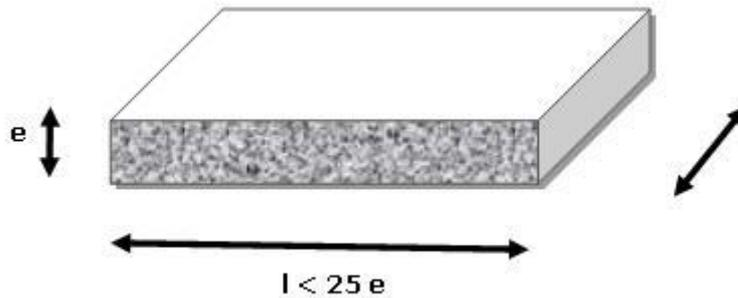
Figure 2: Relations between dimensions of the designed surface
