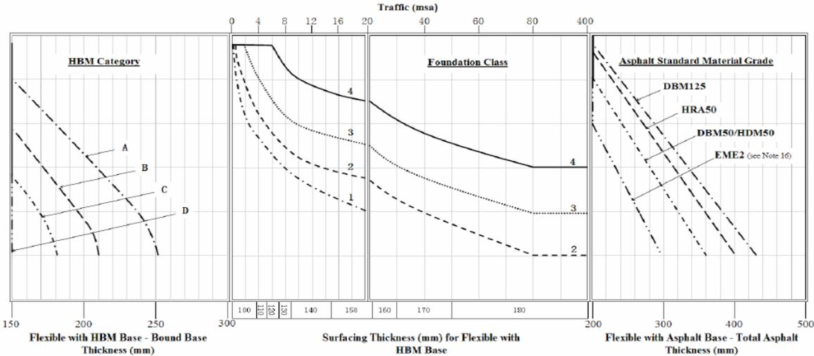
Figure 5: Design Chart for composite construction
