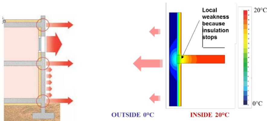
Figure 6: Thermal bridges
