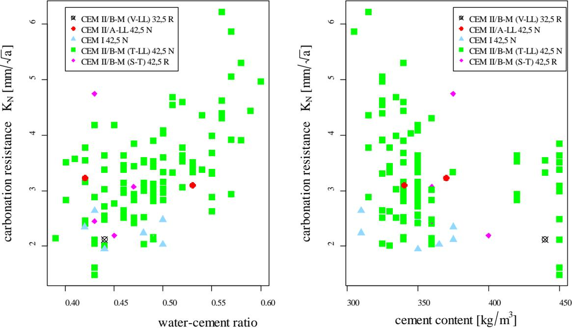
Figure 2: Measured carbonation coefficients  $K_N$  versus water-cement ratio (left) and cement content (right)
