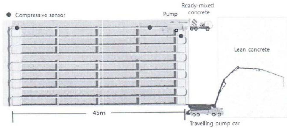
Figure 1: Pumping Test Layout
