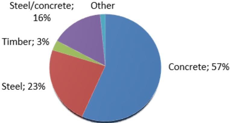
Figure 3: The use of structural materials in housing in Sweden.
