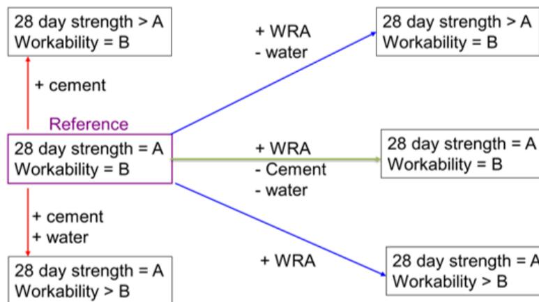
Figure 5: A sketch of different ways of utilizing water reducing agents (WRA) in concrete technology from Rixom and Mailvaganam [14].
