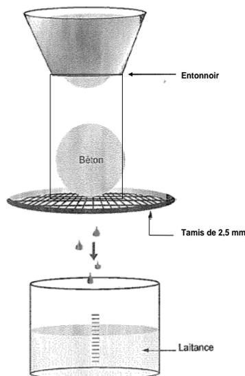
Figure 17: Segregation test scheme
