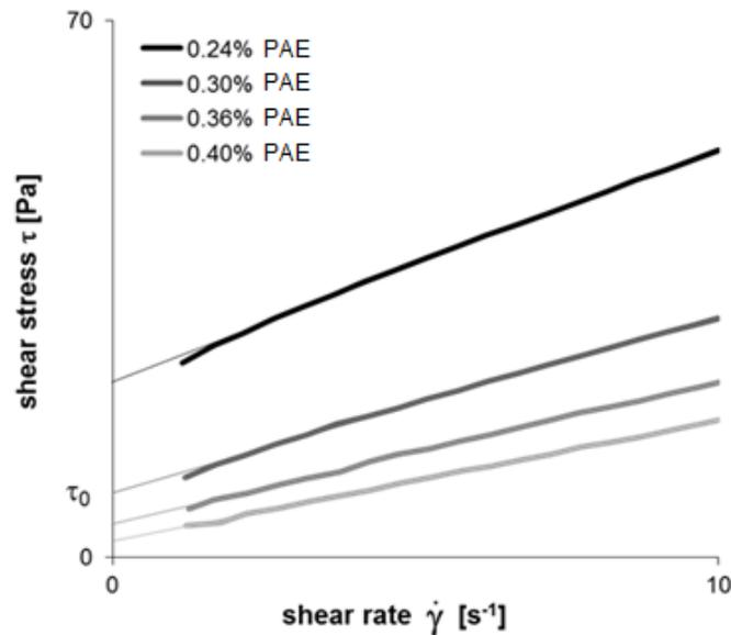
Figure 6: Shear stress of a mortar with different dosages of **PAE** depending on the shear rate.
