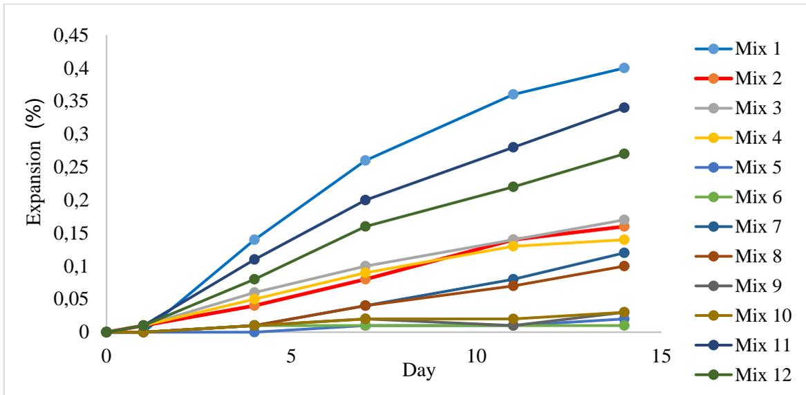
Figure 2: ASTM C 1260 Test results of 12 different mortar mixes
