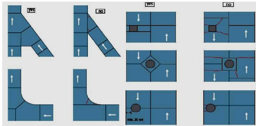
Figure 1: Examples of joint systems and limiting walls
