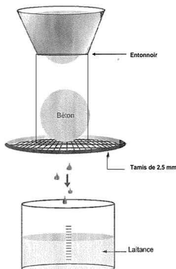
Figure 17: Segregation test scheme
