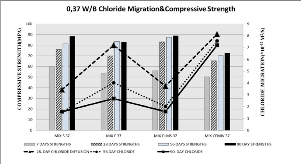
Figure 1: Chloride migration and compressive strength test results for W/B of 0.37
