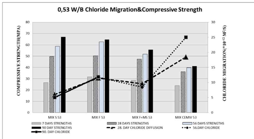
Figure 3: Chloride migration and compressive strength test results for W/B of 0.53
