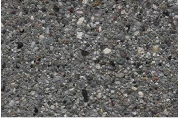
Photo 11: Washed-off surface on aggregate w-8 mm (gravel), grey colouring
