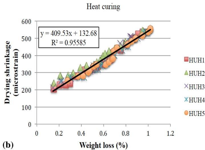
Figure 4: Relationship between drying shrinkage and weight loss, (a) normal curing, (b) heat curing.
