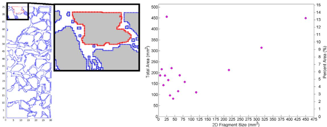
Figure 4: Demonstration of a fragment size analysis conducted on PRC1, 2D fragment size output
