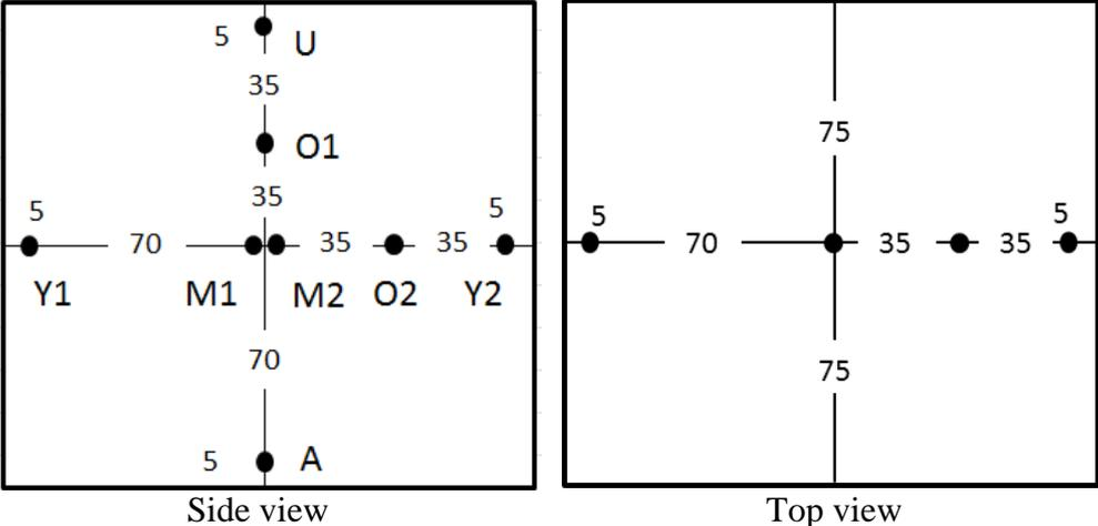
Figure 1 : Temperature measurement locations (distances are given in cm.)
