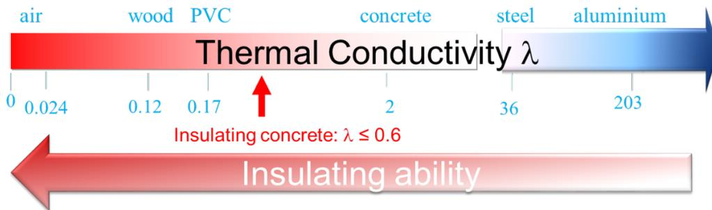
Figure 5: Thermal conductivity of materials
