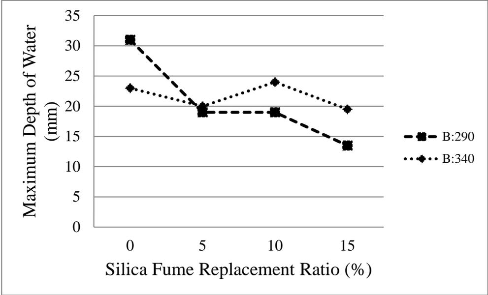
Figure 7: The maximum depths of water ingress measured for concretes.
