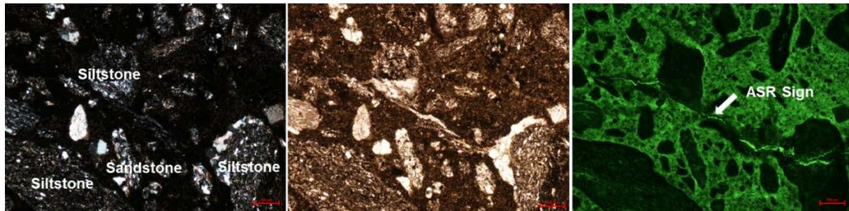
Figure 5: Thin section photos of ASR sign
