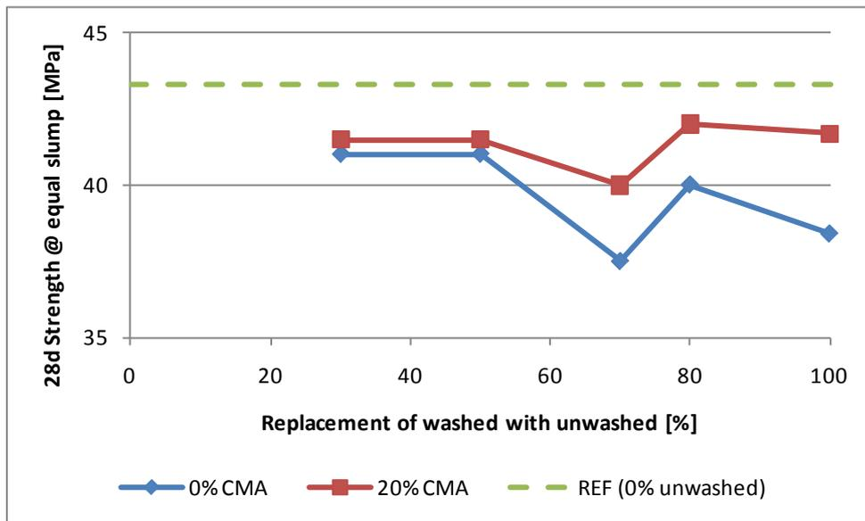
Figure 5: Effect of chemical treatment on strength with increased replacement of washed with unwashed sands
