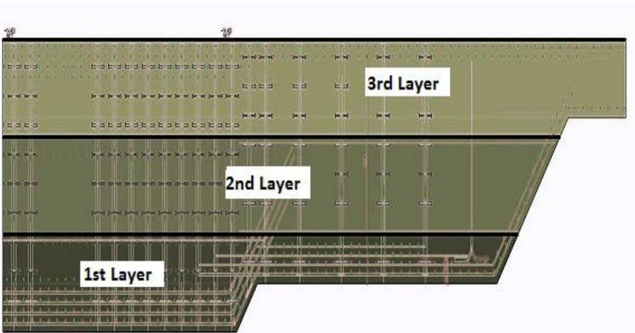
Figure 1: Cross-section of the foundation cast in three layers
