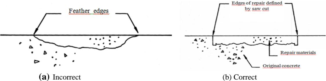
Figure 7: Edges to repairs, the saw cut should be used to avoid feather edges.
