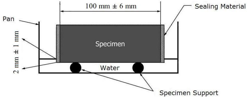
Figure 5: Set up for the capillary test.
