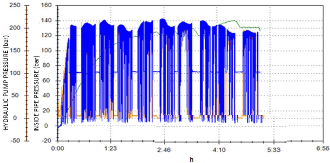
Figure 4: Hydraulic pump pressure and pipe pressure during pumping
