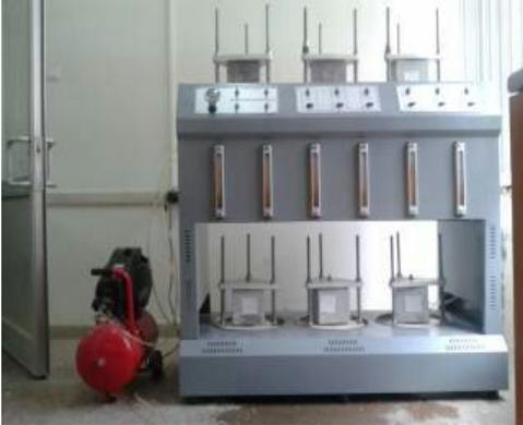
Figure 3: Set up for water ingress.
