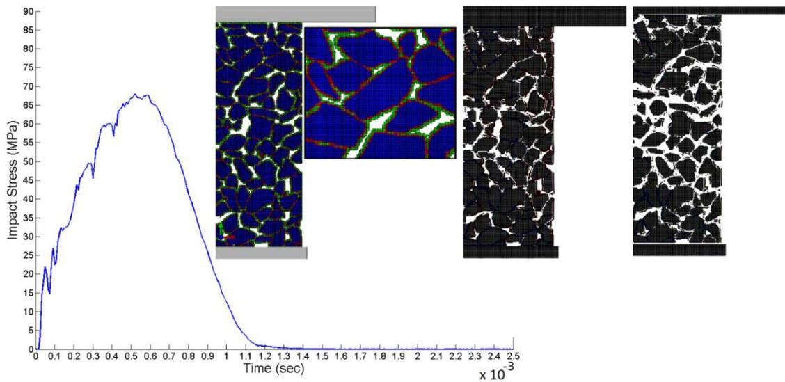
Figure 3: Impact stress time history of PRC1 obtained numerically, the PRC1 finite element mesh and the progress of fragmentation during the analysis (two selected time steps)
