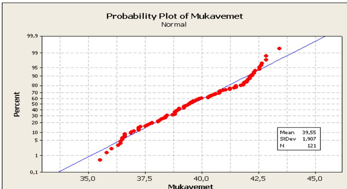
Figure 3: Distribution of compressive strength of the concrete
