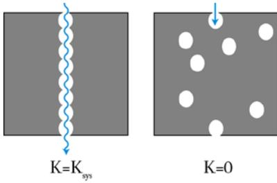
Figure 1: Difference in permeability with the same porosity
