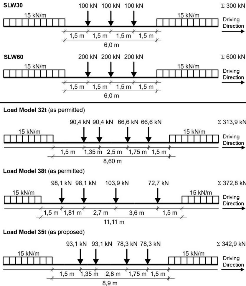
Figure 2: Normative load models of bridge structures and truck mixers [3]
