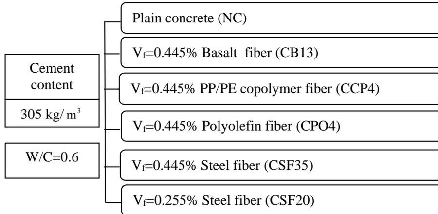
Figure 1: Notation and definition of concrete mixes.
