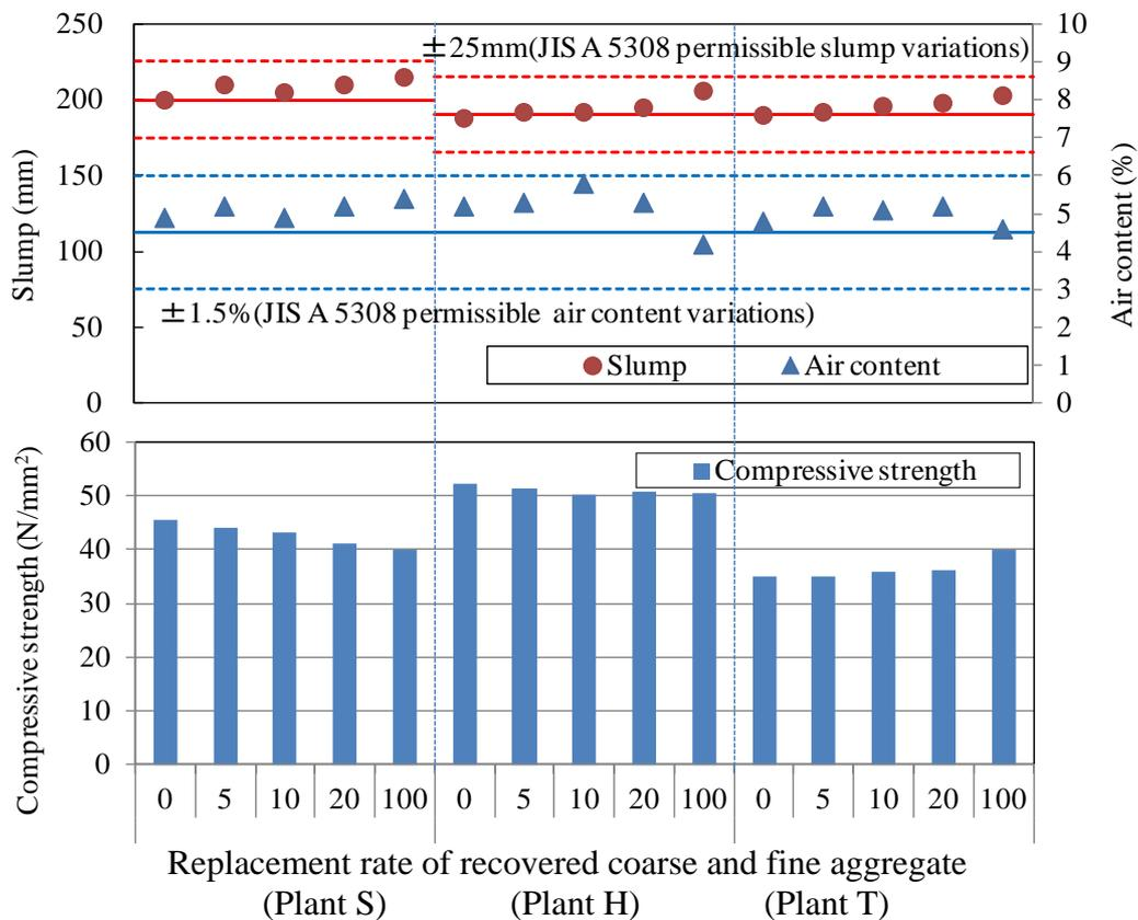
Figure 8: Comparison of concretes properties between recovered aggregate concrete and control concrete
