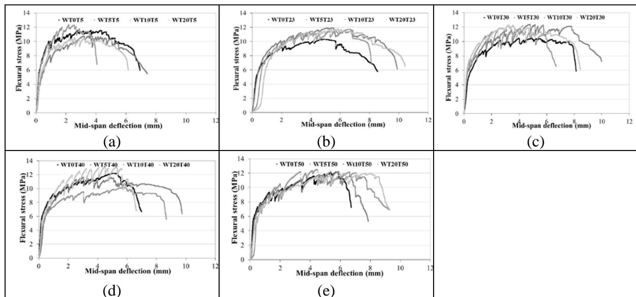
Figure 2: Flexural stress mid span deflection graphs (a) 5 °C (b) 23 °C (c) 30 °C (d) 40 °C (e) 50 °C
