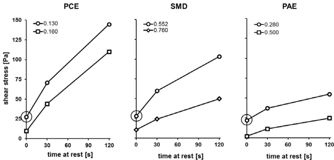
Figure 4: Correlation between shear stress and time at rest for different superplasticizer types, applied at two different dosages
