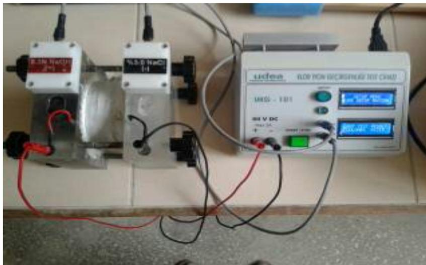
Figure 2: Set up for rapid chloride permeability test.
