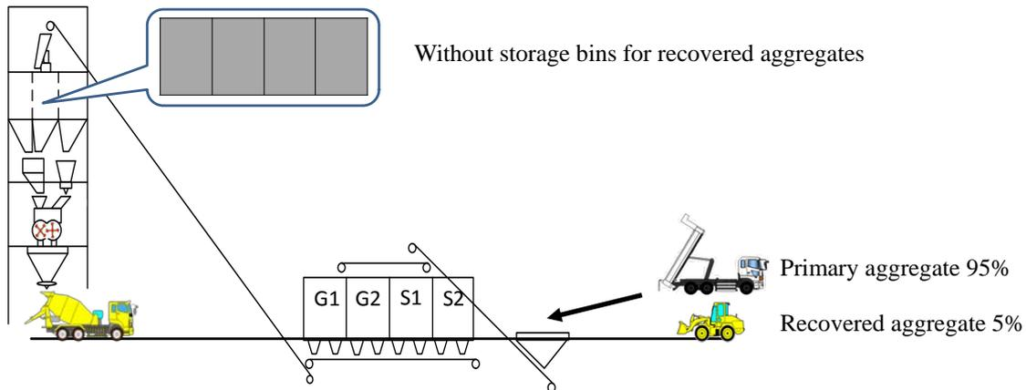
Figure 4: Hopper supply procedure (Method A)
