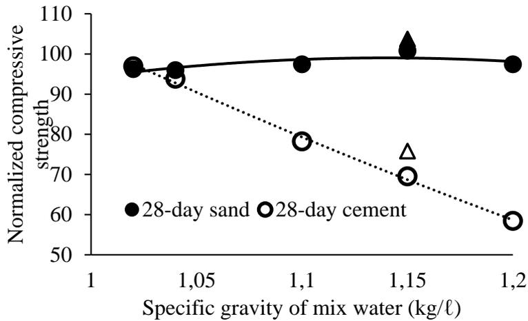
Figure 3: Normalized compressive strength at the age of 28 days
