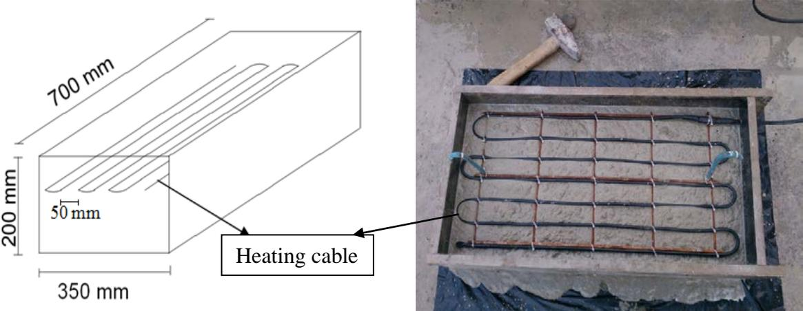
Figure 2: Heating cable positioned into sample prior to testing.
