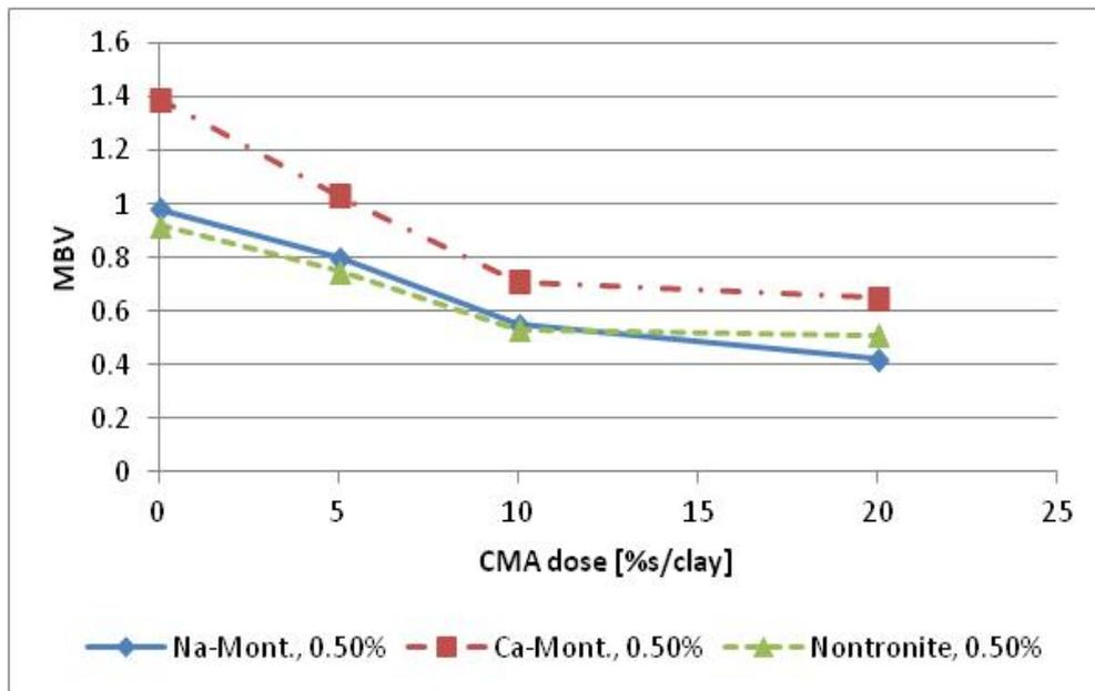
Figure 3: Effect of a CMA on the MBV
