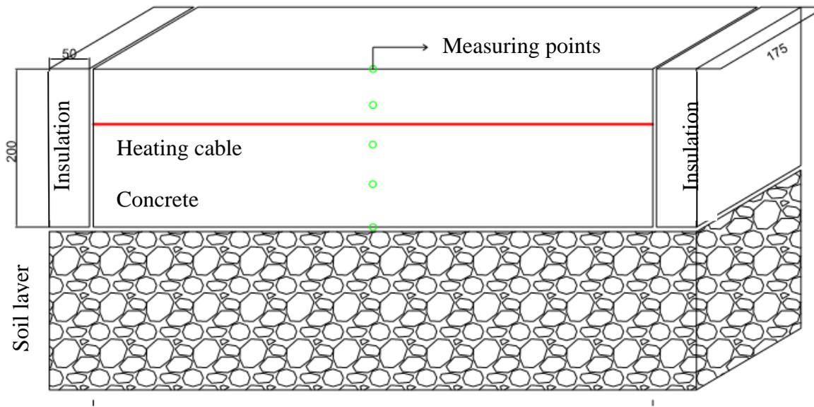
Figure 3: Concrete sample on top of the soil inside the freezer.
