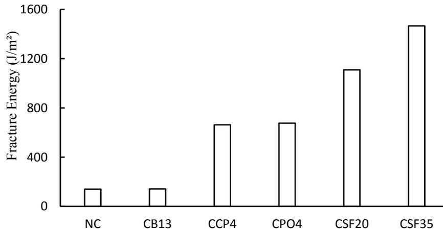
Figure 5: Fracture energy of plain and fiber reinforced and plain concretes.
