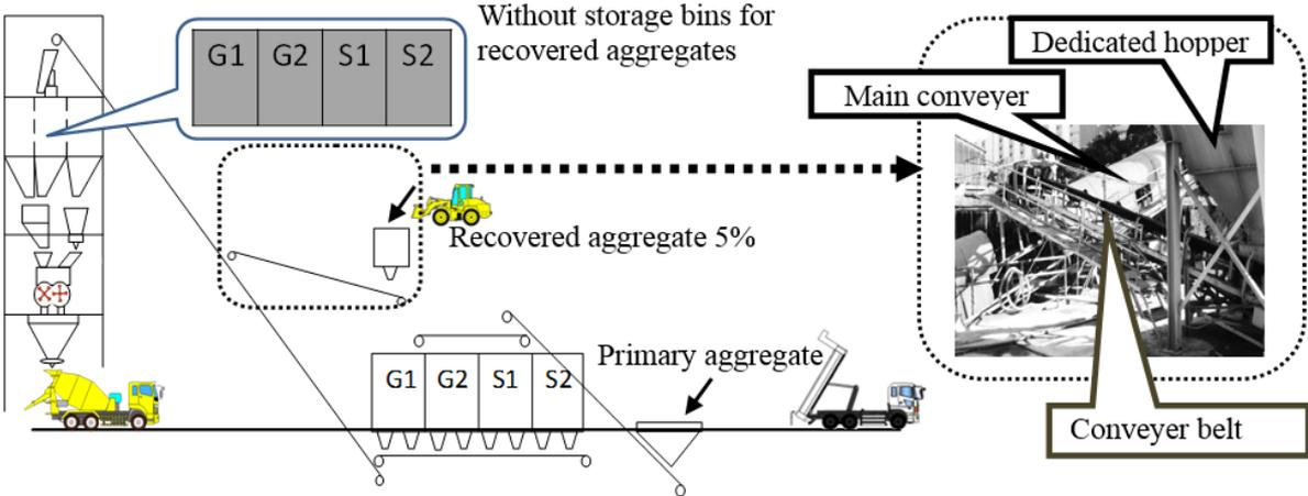
Figure 3: Conveyer belt supply procedure (Method A)
