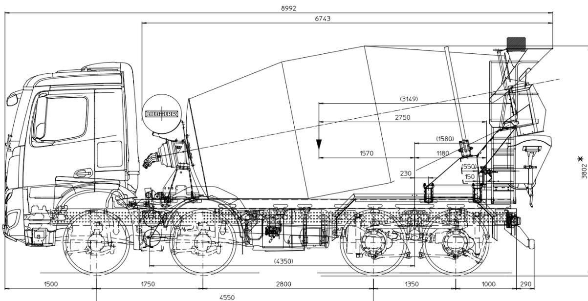
Figure 1: Model of a 35t four-axle truck mixer with modified wheelbase [1]
