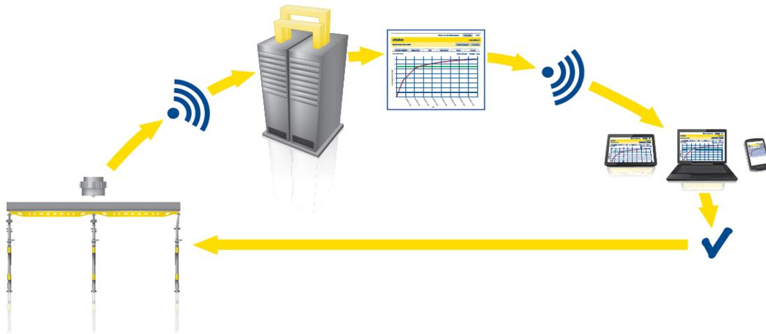
Figure 3: Process of concrete monitoring system
