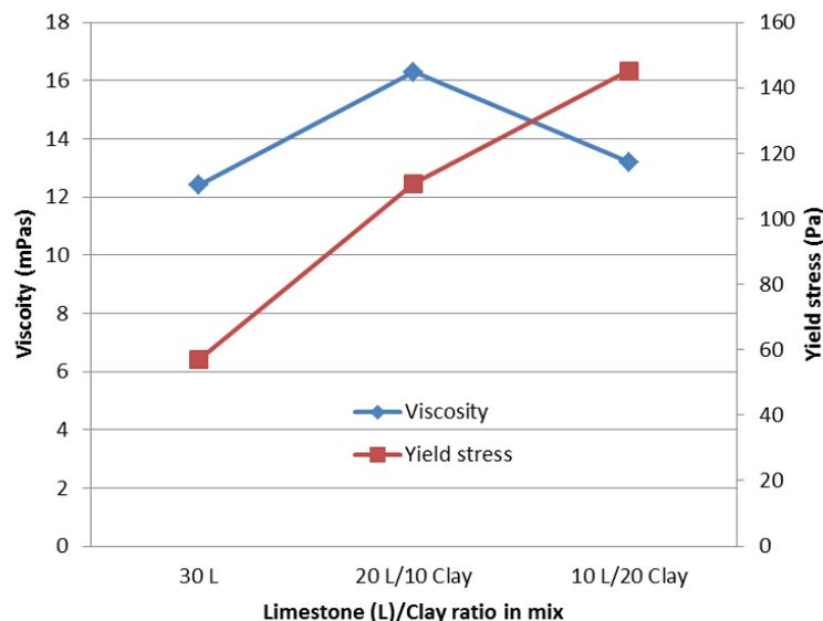
Figure 1: The viscosity and yield stress of SCC where limestone powder (L) is increasingly replaced by calcined blue clay (Clay) from Justnes et al. [1].
