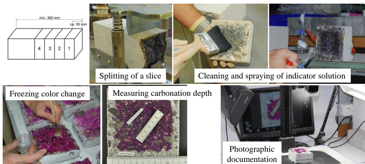
Figure 1: Testing procedure according to SIA 262-1/Appendix I [1]
