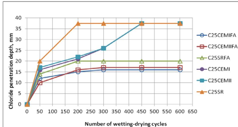
Figure 3: Chloride penetration depths for Class C25/30 concretes.
