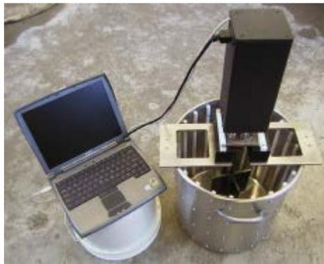
Figure 1: RHM 3000 ICAR Rheometer
