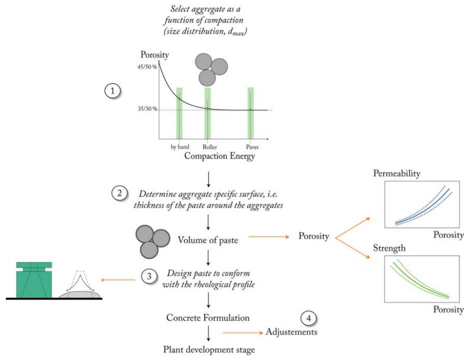
Figure 7: Permeable concrete design scheme
