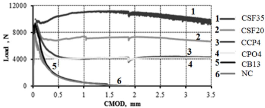
Figure 7: CMOD-load graphics of fiber reinforced and plain concretes.
