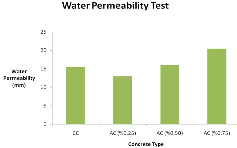
Figure 6: Graphical display of the test results of the water permeability
