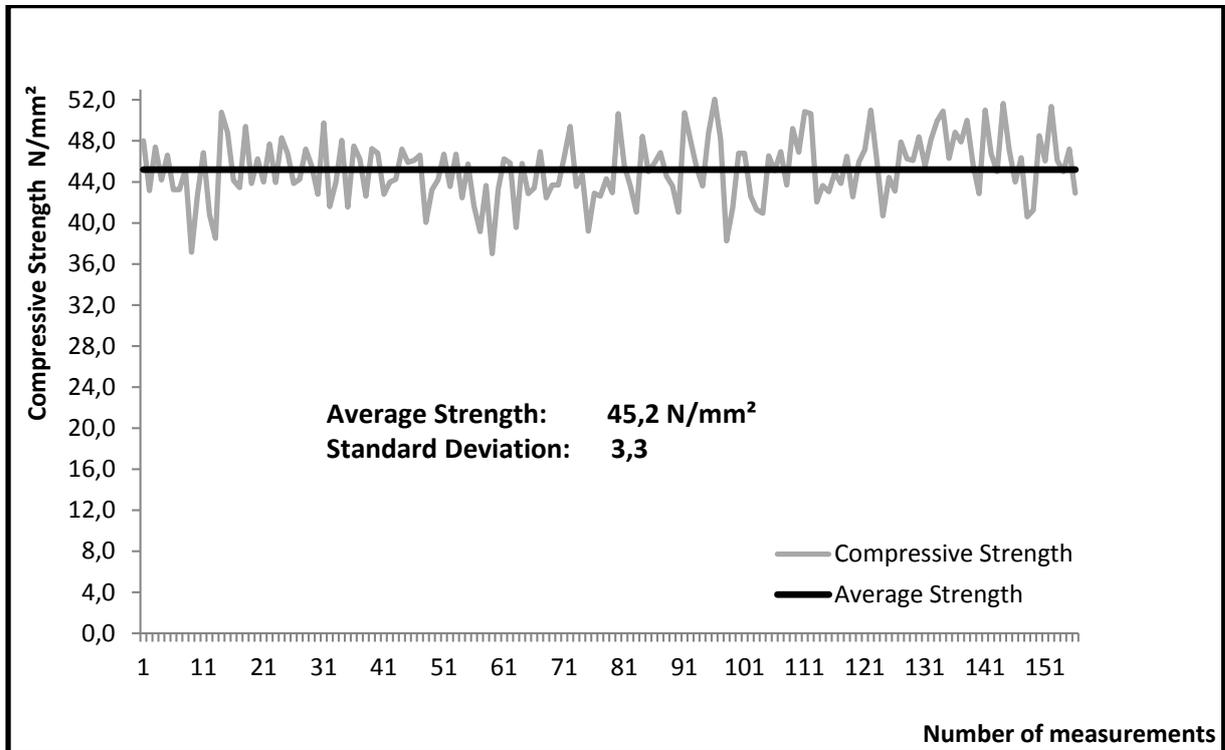
Figure 5: Compressive strength analysis of C30-C37 Concrete with CLR-S
