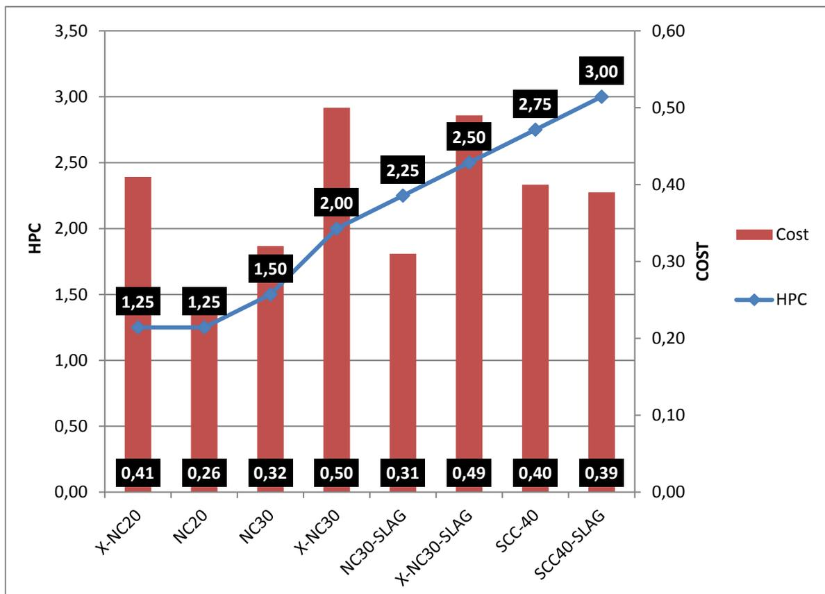
Figure 2: Cost and HPC for tested mix designs
