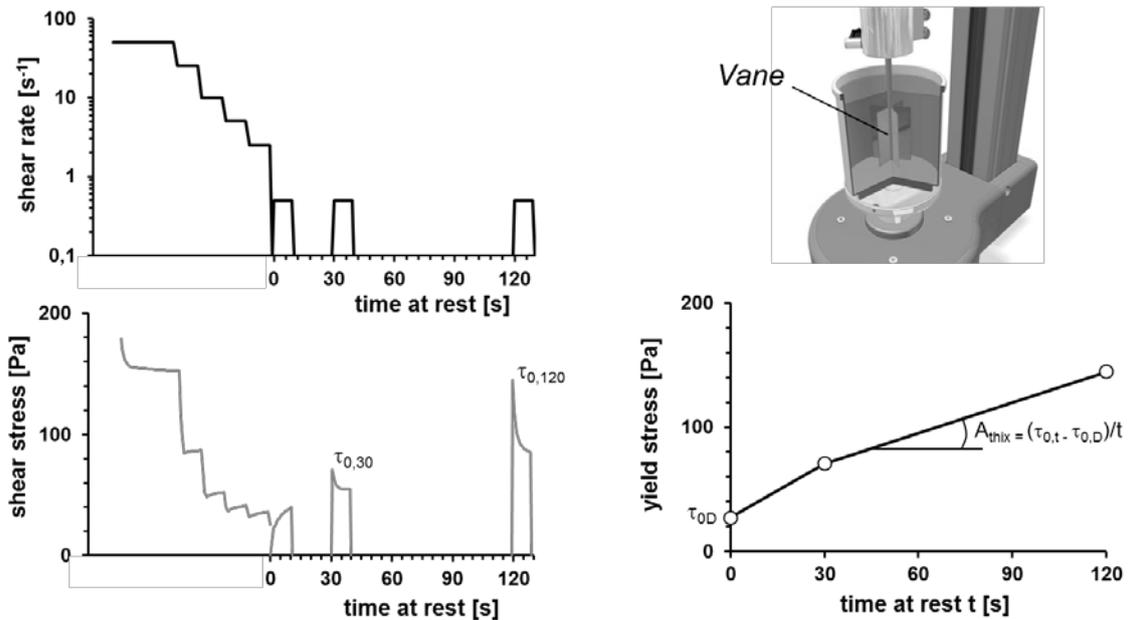
Figure 9: Shear rate profile for detection of shear stress depending on time at rest.
