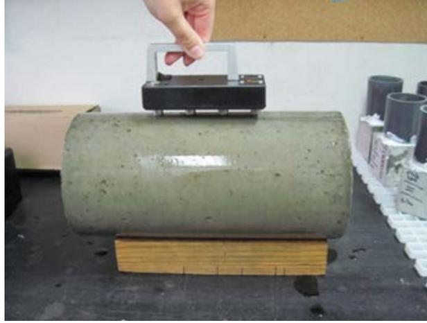
Figure 3: Resistivity measured with a four-point resistivimeter.
