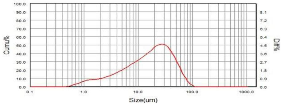
Figure 1: Particle size graphic of K-1 cement
