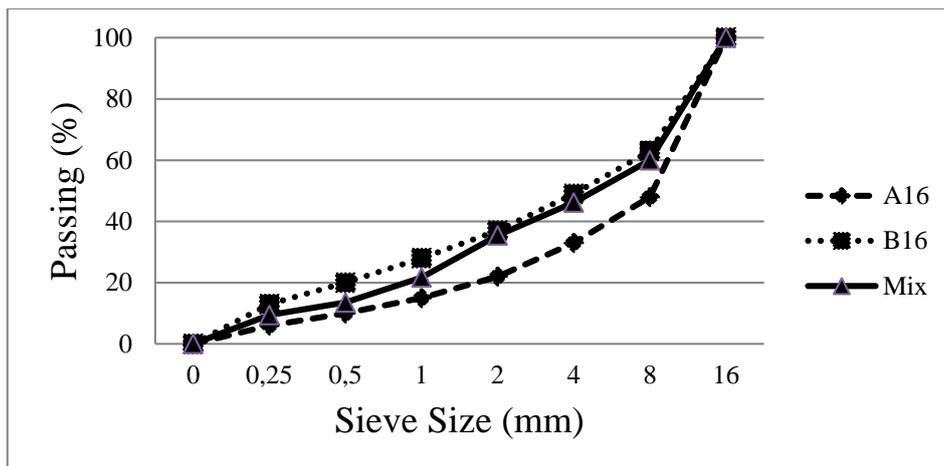
Figure 1: Gradation of the aggregate mix and the reference curves.
