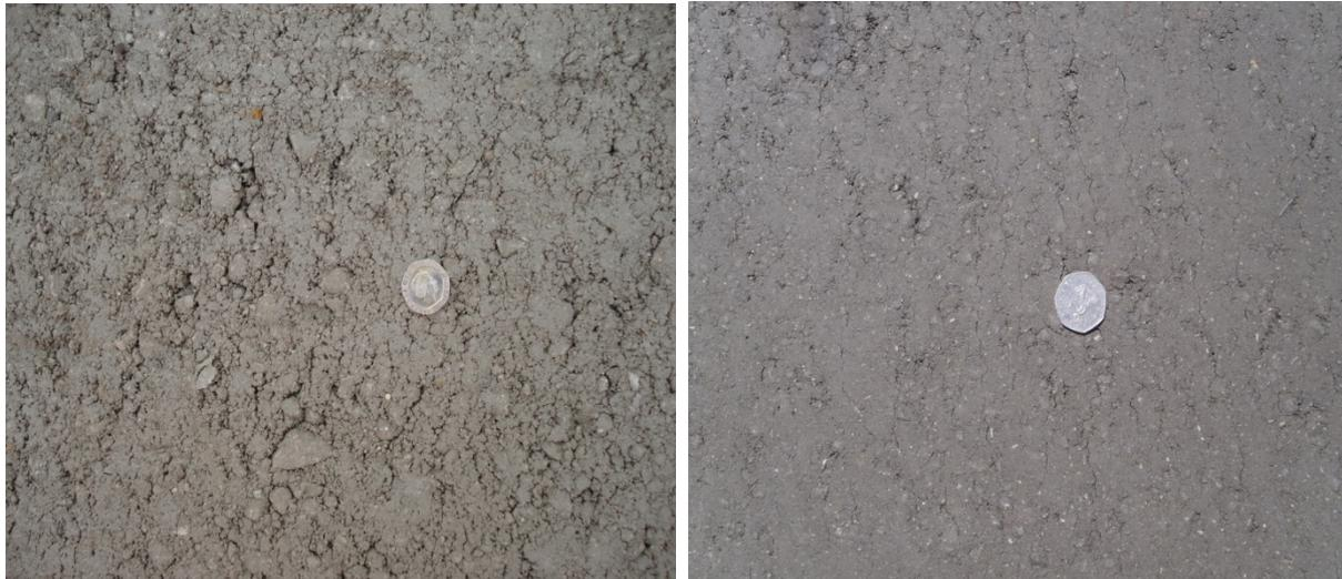
Figure 1: Typical surface finish with 20mm (left) and 10 mm (right) maximum aggregate size
