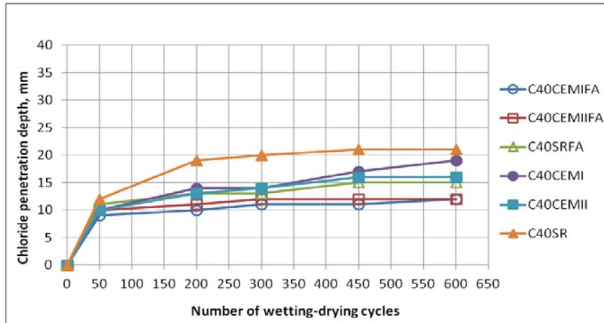
Figure 4: Chloride penetration depths for Class C40/50 concretes.
