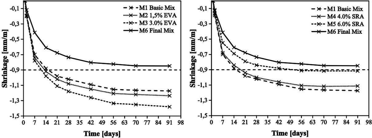
Figure 3: a) measured shrinkage for varying concentrations of the copolymer used; b) measured shrinkage for varying concentrations of the shrinkage reducing admixture used
