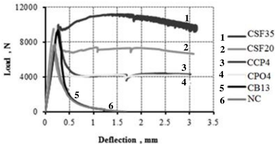
Figure 4: Load versus deflection curves of fiber reinforced and plain concretes.
