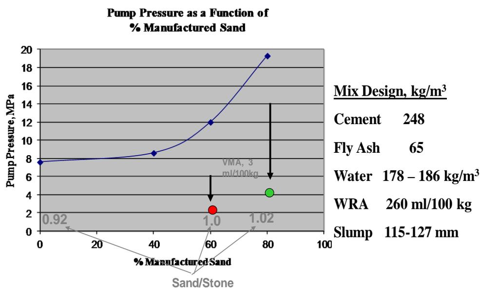
Figure 2: Effect of VMAs and Manufactured Sands on Pump Pressure
