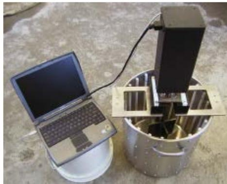
Figure 1: RHM 3000 ICAR Rheometer
