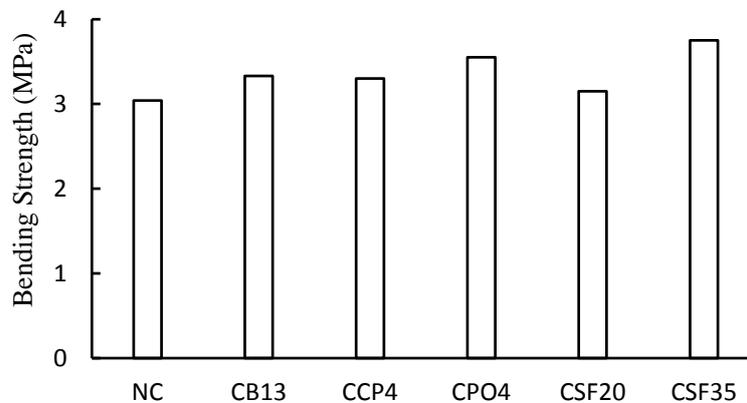
Figure 6: Bending strength of fiber reinforced and plain concretes.
