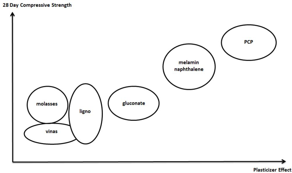
Figure 1: Raw material effects on 28 day compressive strength [2].
