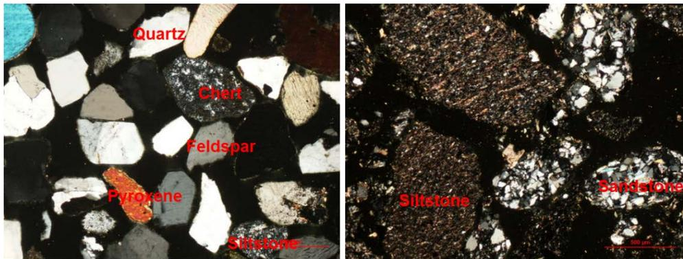
Figure 1: Thin section photos of F1-ÇATALCA natural sand and F2-CENDERE crushed sand. Thin section photos were taken with x 50 magnification.
