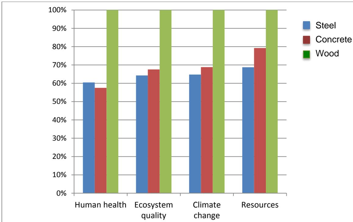
Figure 4: Transportation and construction phase - impact categories
