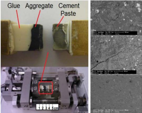
Figure 1: Meso-scale composite ITZ sample, meso-scale testing set-up and ESEM images of the aggregate surfaces of ITZ samples after testing
