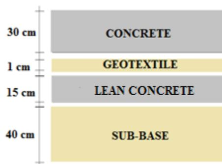
Figure 2: Section of the pavement
