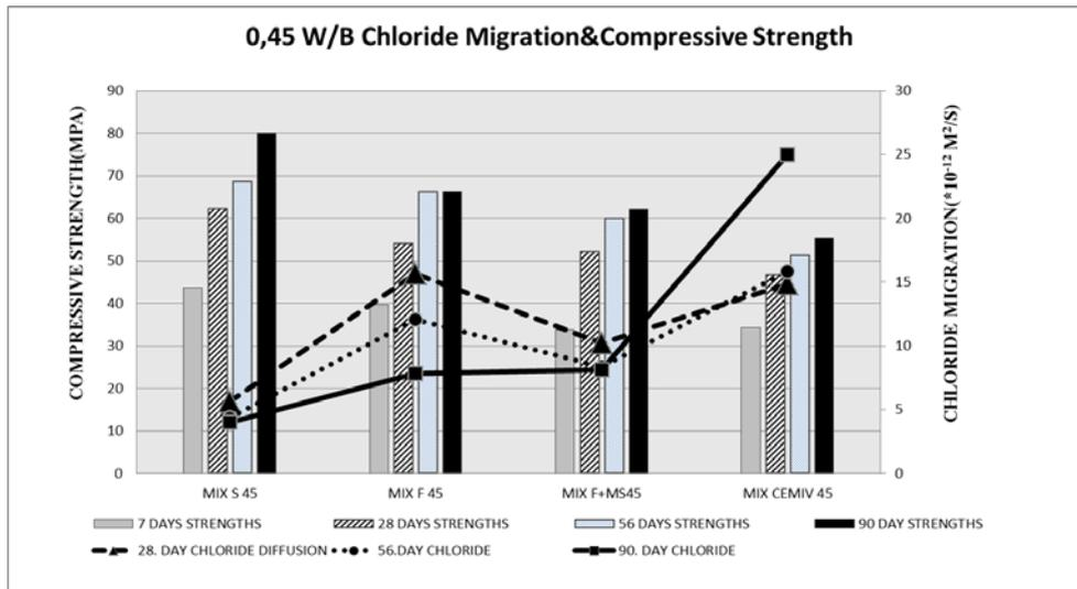
Figure 2: Chloride migration and compressive strength test results for W/B of 0.45
