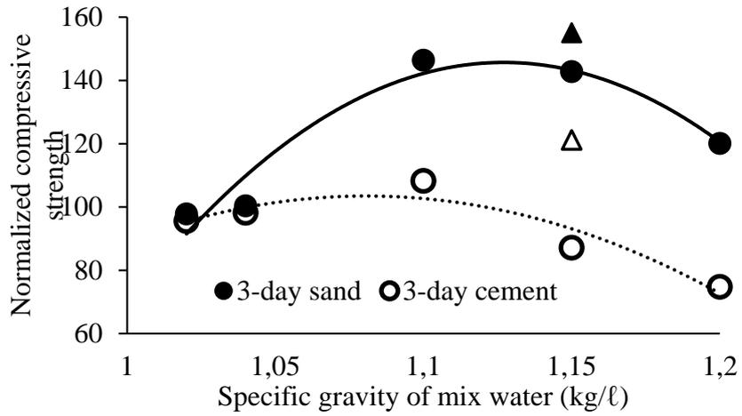
Figure 1: Normalized compressive strength at the age of 3 days (Triangle points correspond to concretes with modified workability)
