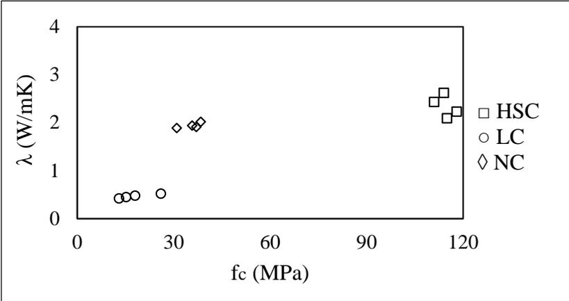
Figure 2: Comparison of compressive strength-thermal conductivity coefficient relationship of series
