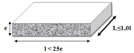
Figure 4: Scheme of designed dimensions
