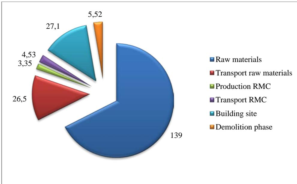
Figure 4: separate contributions for warm technique (kg CO<sub>2</sub>/m<sup>3</sup>)
