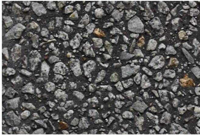
Photo 13: Washed-off surface on aggregate 2-16 mm (granite grit) and black-coloured mortar
