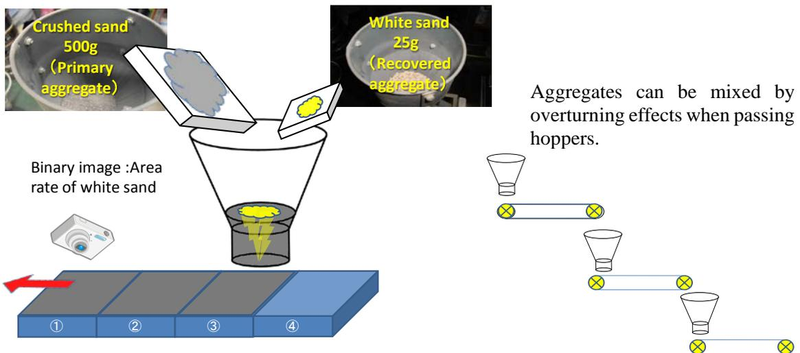
Figure 6: Mixing of aggregate by overturning effects
