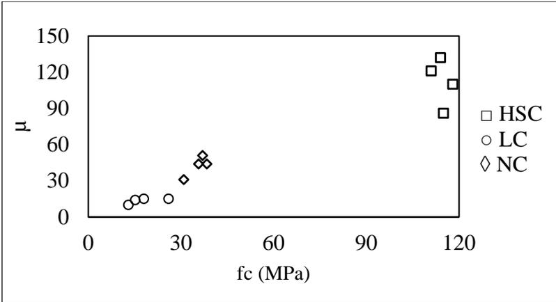
Figure 1: Comparison of compressive strength-vapor diffusion resistance factor relationship of series
