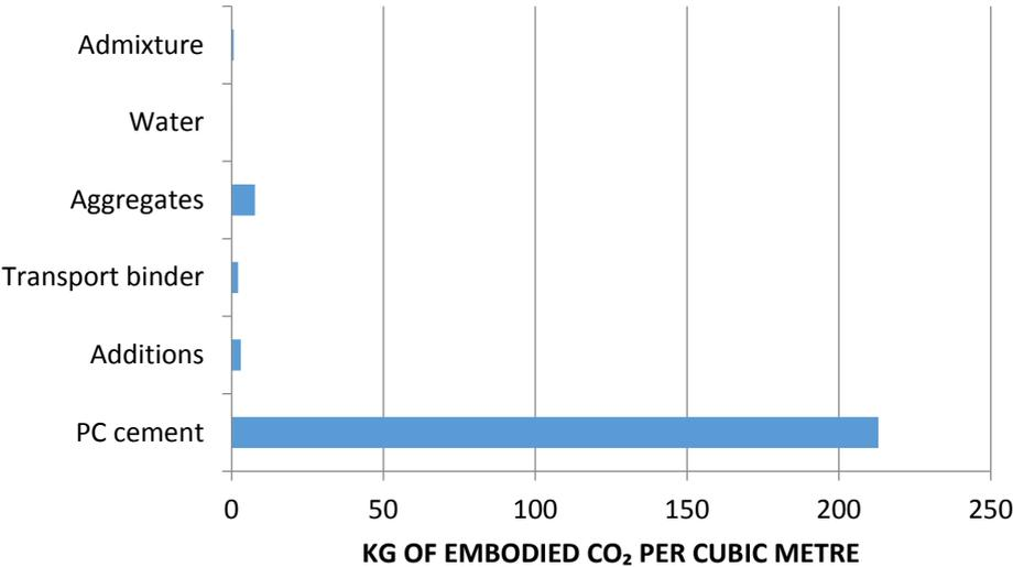
Figure 1: Embodied carbon dioxide per cubic metre of average UK concrete
