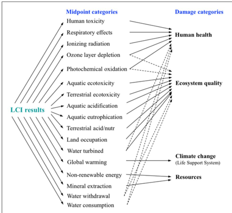
Figure 2: Impacts and damage categories scheme
