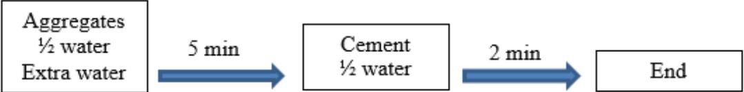
Figure 3: Followed two-staged mixing method
