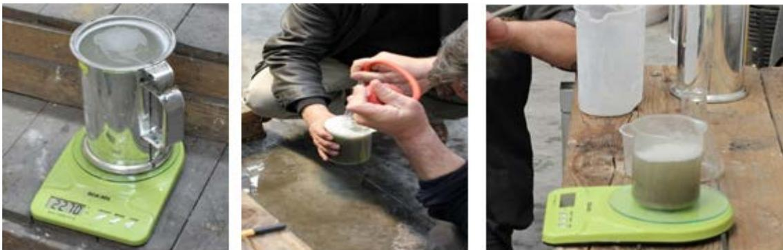
Figure 1: Density measurement by weighing
