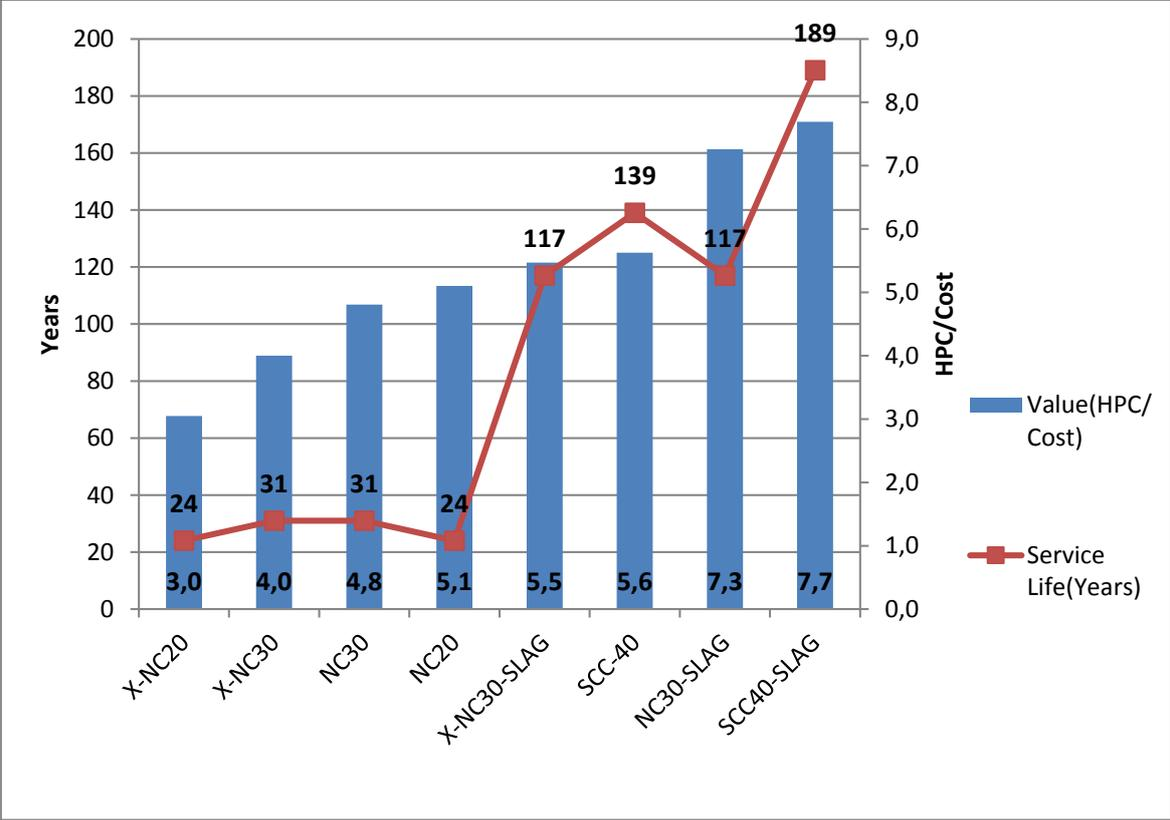
Figure 3: Service life and value for tested mix designs
