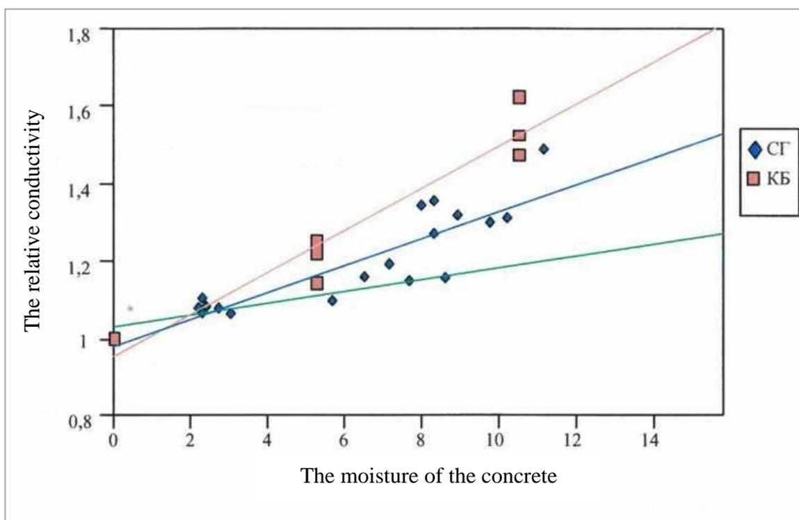
Figure 1: Effect of Moisture Content on the Coefficient of Relative Thermal Conductivity of Lightweight Concrete on GPG
