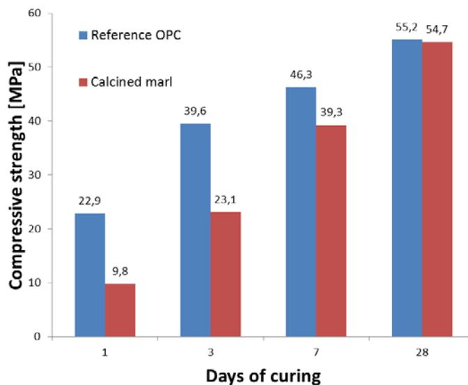
Figure 3: Compressive strength of mortars with 0 (reference) and 50 % replacement of cement by calcined marl cured for 1, 3, 7 and 28 days [2].
