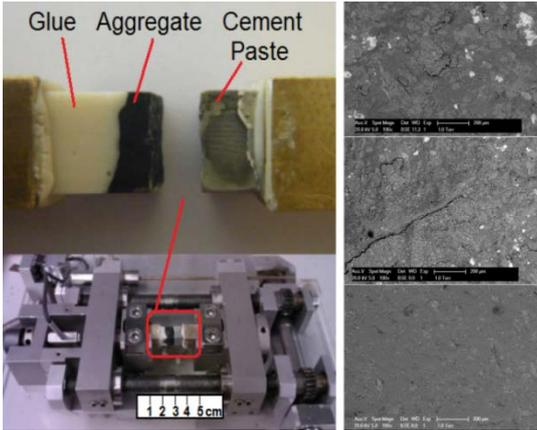
Figure 1: Meso-scale composite ITZ sample, meso-scale testing set-up and ESEM images of the aggregate surfaces of ITZ samples after testing
