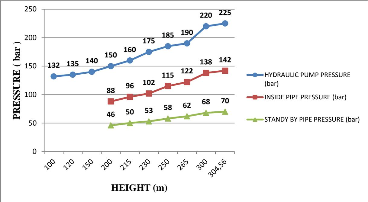
Figure 3: Height vs Pressure Chart
