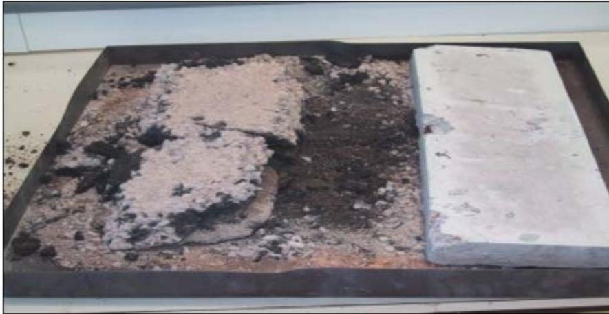
Figure 1: Comparison of specimens of asphalt (left) and concrete (right) after heating to 750°C [3]
