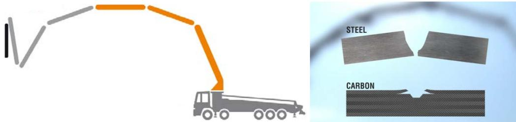
Figure 8: Carbon fiber versus steel. No cracks on placing booms
