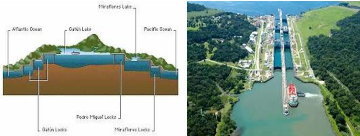
Figure 1: Profile of the height of the inland Gatun lake and the need to build locks (right part) for the navigation.
