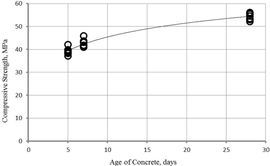
Figure 5: In normal weather conditions, relation between cylinder compressive strength and age of concrete for Mix 3
