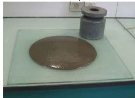
Figure 11: Mini stożek (Mini Slump)
