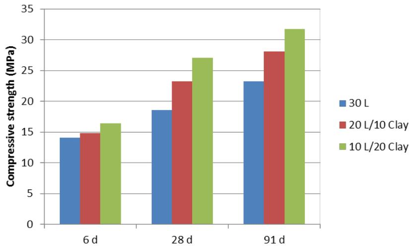
Figure 2: Compressive strength evolution of SCC where limestone powder (L) is replaced by calcined blue clay (Clay) from Justnes et al. [1].
