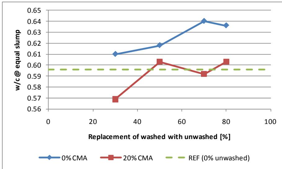
Figure 4: Effect of chemical treatment on w/c with increased replacement of washed with unwashed sands.
