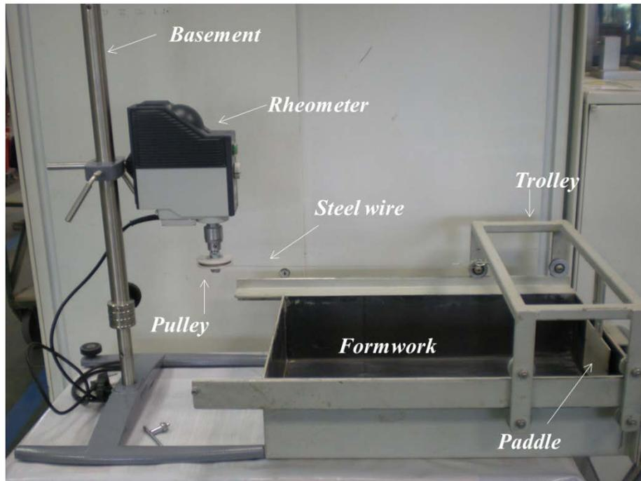
Figure 2: Placing Simulation Tool
