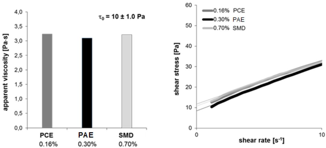
Figure 8: Apparent viscosity at constant yield stress
