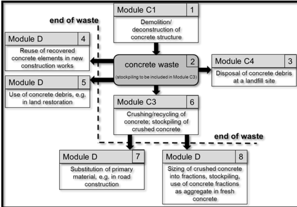
Figure 3: Typical processes at the end-of-life of concrete and concrete products and their assignment to the life cycle modules C1-C4 and D (transport processes not shown)
