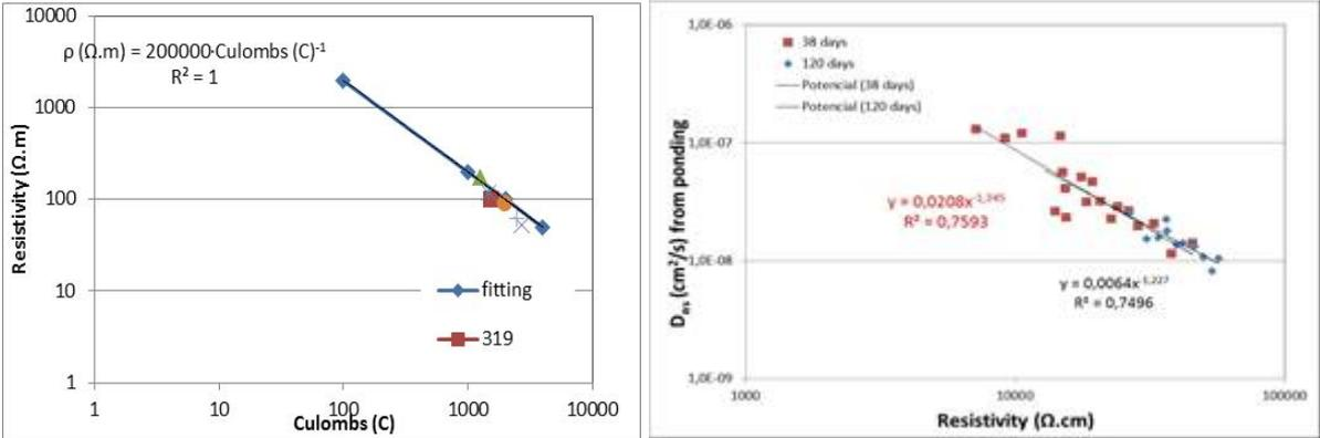
Figure 5: Left- relationship between electrical charge in coulombs and resistivity; and right- relationship between resistivity and the 38- and 120-day apparent diffusion coefficients.
