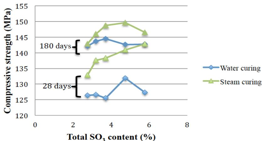
Figure 1: Effect of sulfate content on the compressive strength of UHPFRC.
