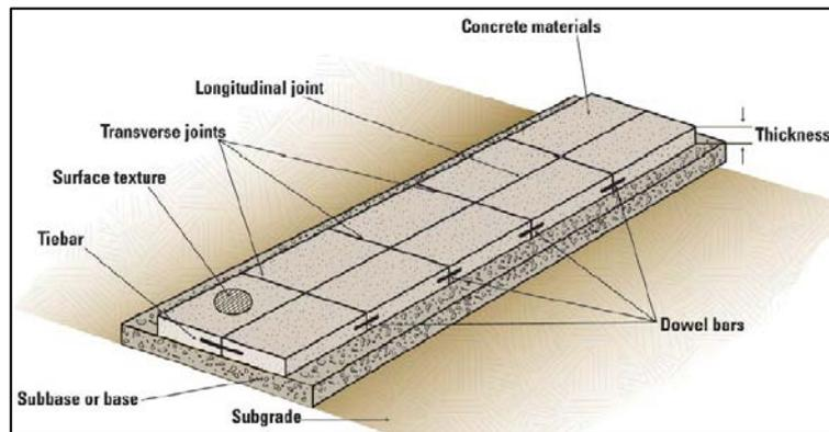
Figure 3: Joint Plain Concrete Pavement (JPCP)
