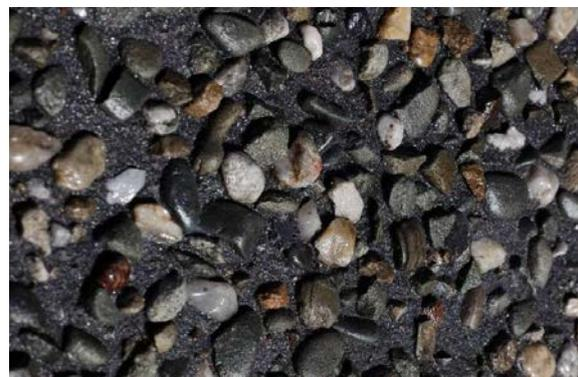
Photo 10: Washed-off surface on aggregate 8-16 mm (gravel) and black colouring.
