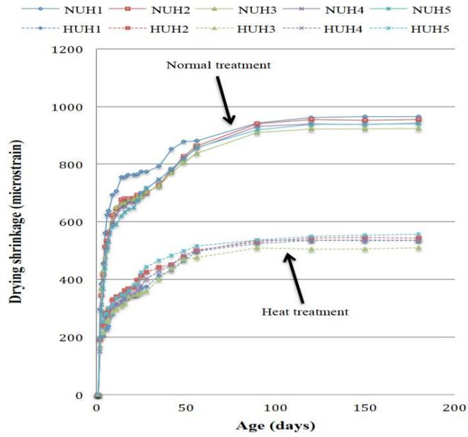
Figure 2: Drying shrinkage of UHPFRC.
