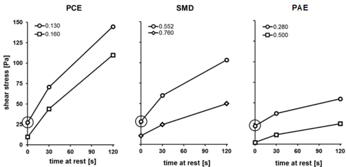
Figure 10: Correlation between shear stress and time at rest for different superplasticizer types
