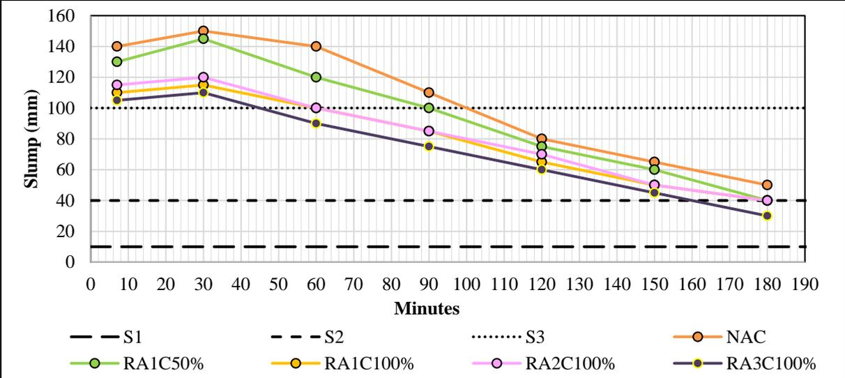
Figure 4: Slump test over time
