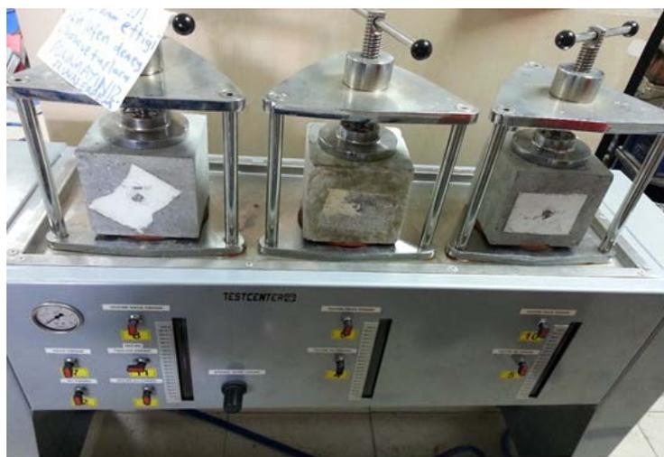
Figure 3: Water permeability testing apparatus
