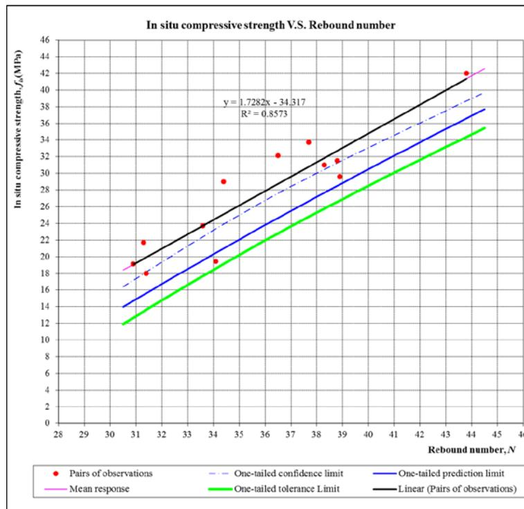
Figure 2: Illustration showing why the 90% confidence limit is not safe (Figure by courtesy of INEC)
