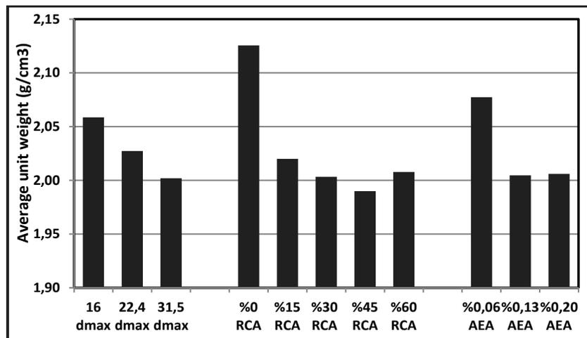
Figure 2: Average unit weight values by parameters
