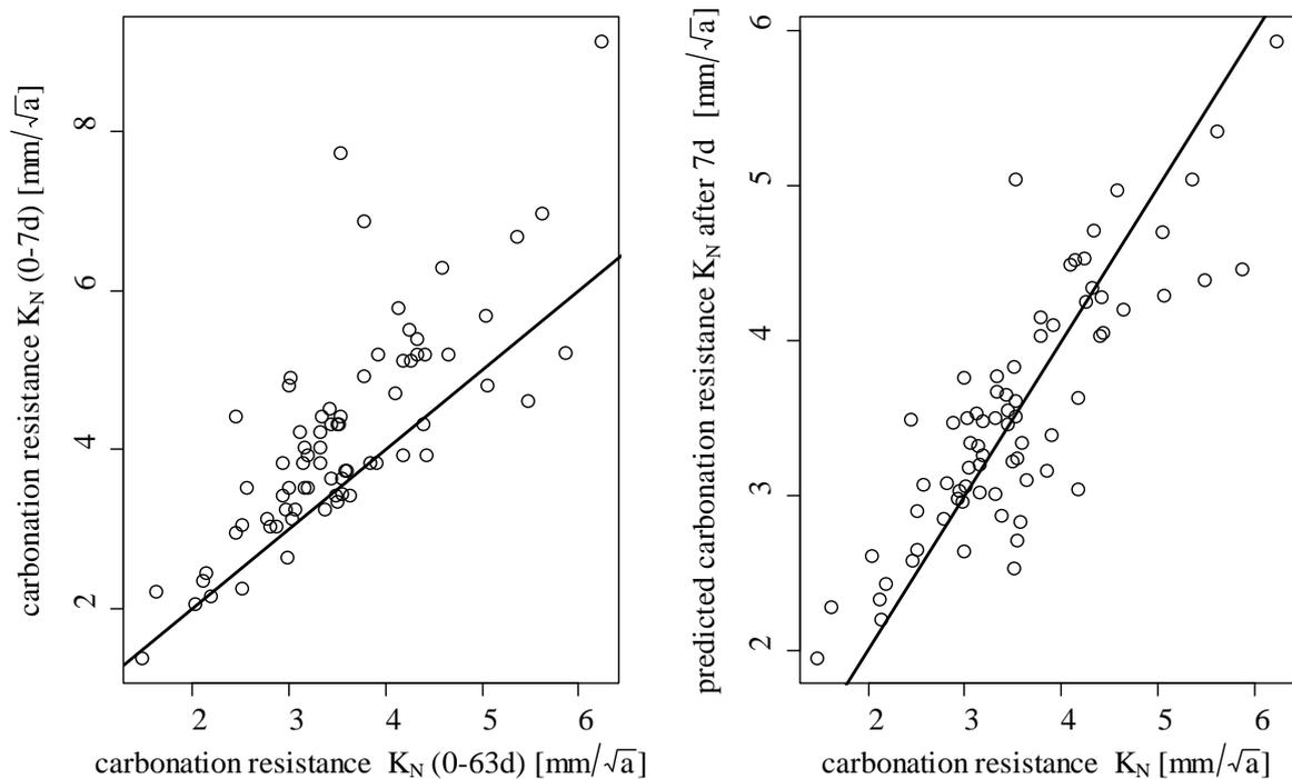
Figure 3: In the left figure the calculated carbonation resistances using 0-7d vs 0-63d values are shown. In the right figure the predicted carbonation coefficient  $K_N$  (with a model using 0-7d accelerated carbonation depth values and water-cement ratio) versus the standard carbonation coefficient  $K_N$  (using as described 0d, 7d, 28d and 63d carbonation depth values)
