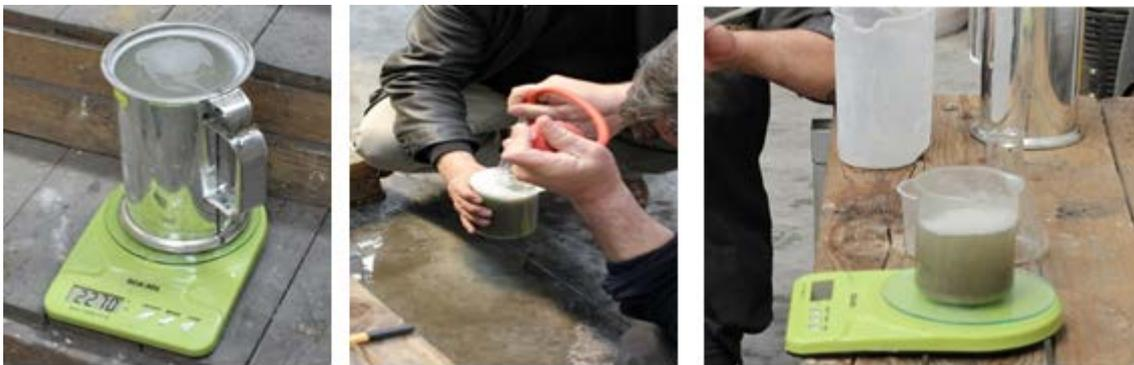
Figure 1: Density measurement by weighing
