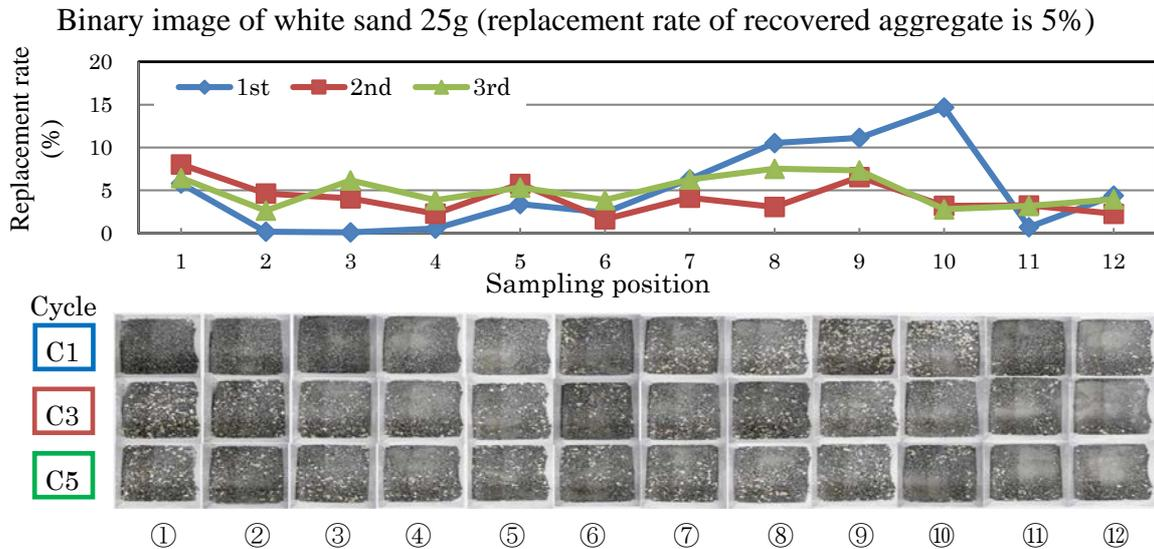
Figure 5: Binary image of recovered aggregate in white at a replacement rate of 5%
