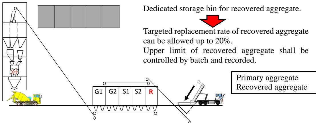
Figure 7: Case of using dedicated storage equipment (Method B)
