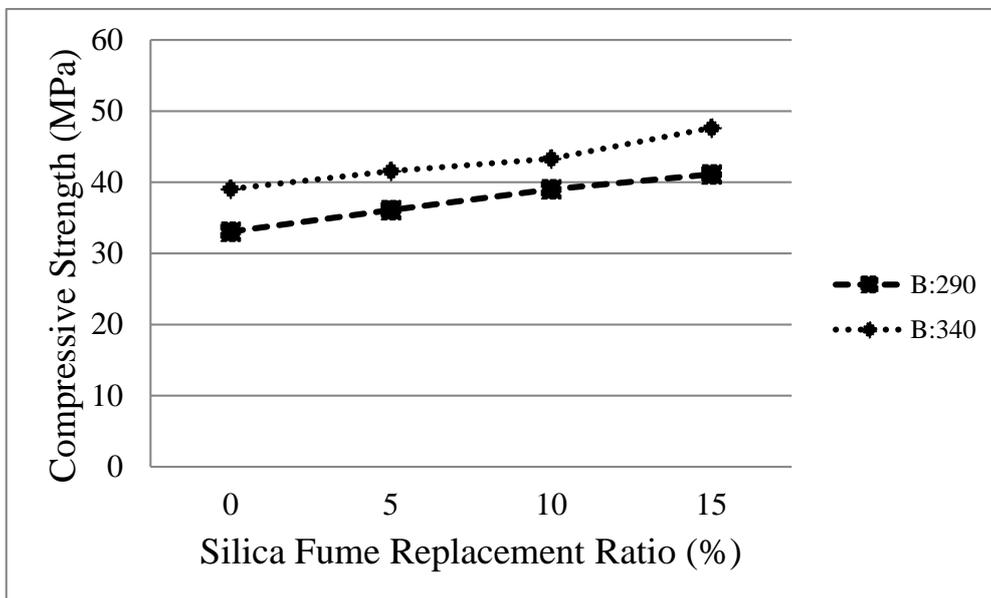
Figure 9: Compressive strengths versus silica fume replacement.
