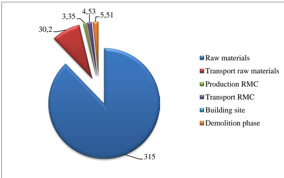
Figure 5: separate contributions for cold technique (kg CO<sub>2</sub>/m<sup>3</sup>)
