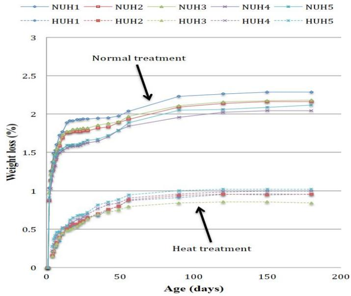
Figure 3: Weight loss of UHPFRC.
