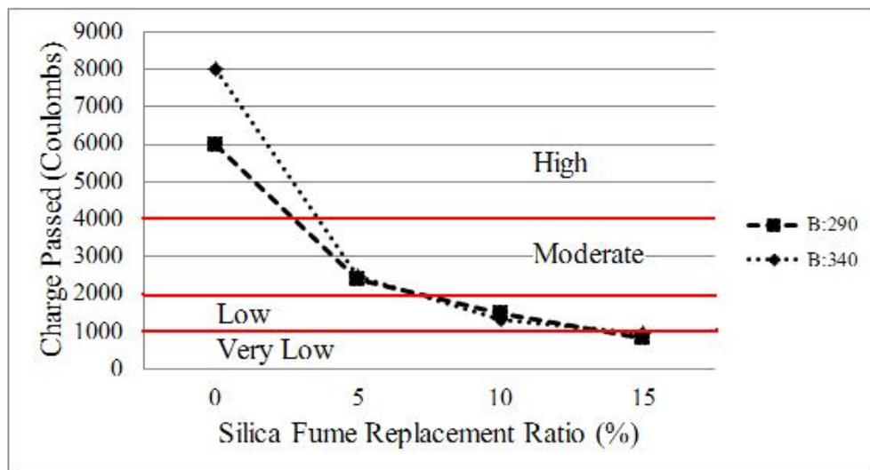
Figure 6: Rapid chloride permeability profiles for concretes.
