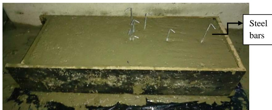
Figure 1: Placement of steel into the concrete sample
