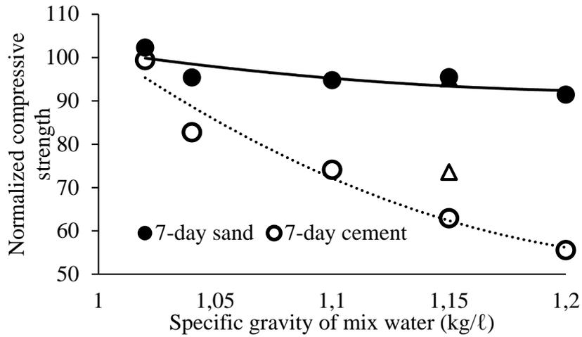
Figure 2: Normalized compressive strength at the age of 7 days
