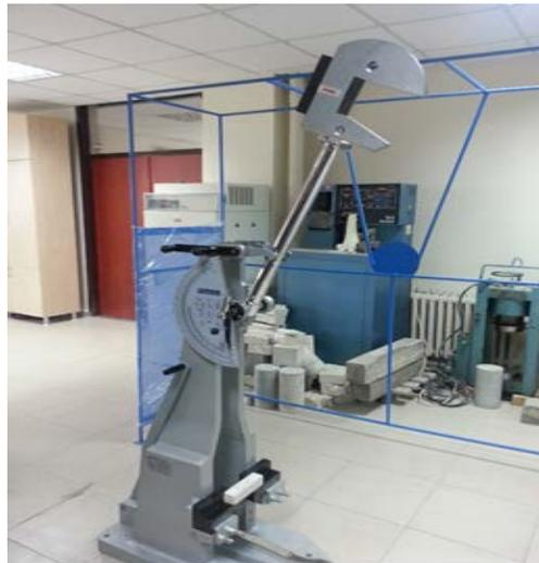
Figure 2: Charpy testing apparatus
