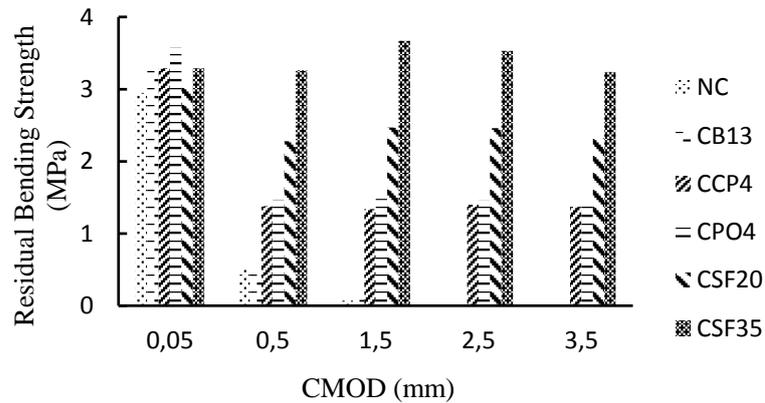
Figure 9: The residual strengths-CMOD of fiber reinforced and plain concretes.
