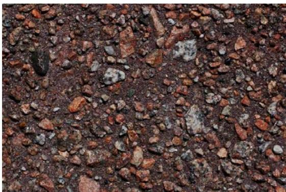
Photo 9: Washed-off surface on aggregate up to 16 mm (granite grit) and brown-coloured mortar.
