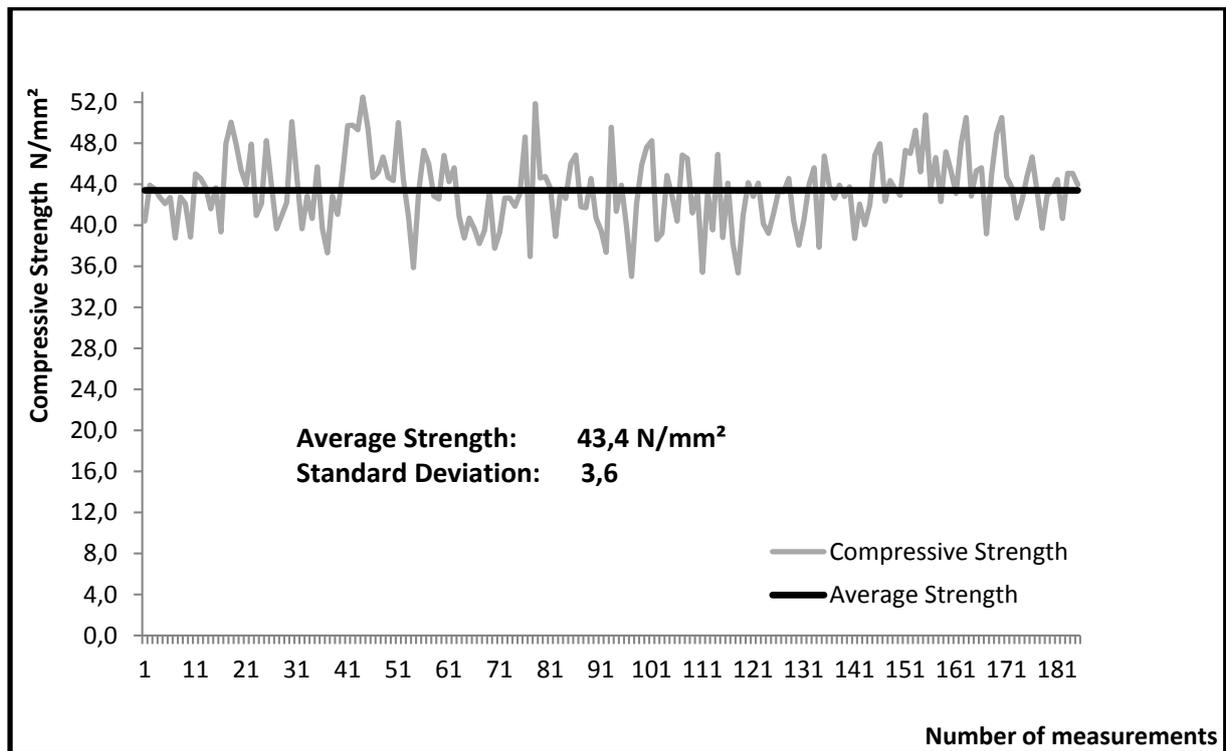
Figure 4: Compressive strength analysis of C30-C37 Concrete with presently used methods)
