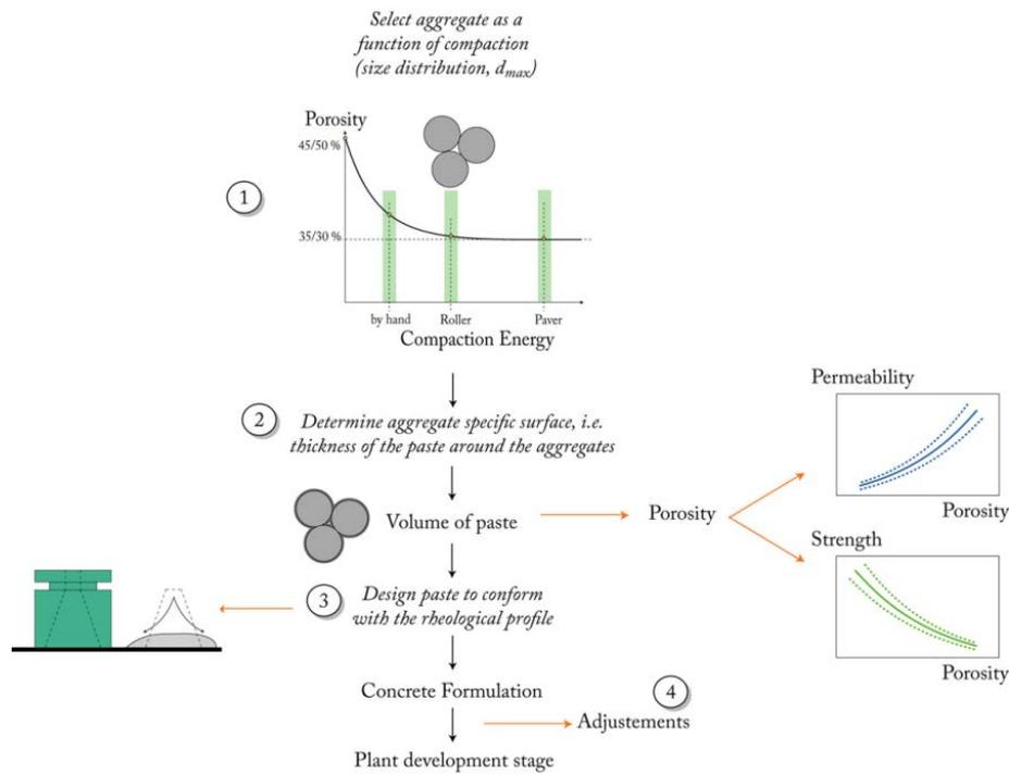
Figure 7: Permeable concrete design scheme
