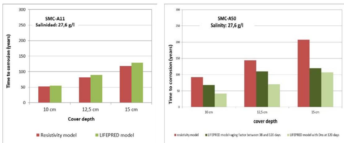
Figure 6: Left- comparison of the LIFEPRED and resistivity models for mix A11; right- comparison for mix A50 of resistivity model to LIFEPRED using the aging factor between 38/120-days and LIFEPRED using the  $D_{ns}$  value obtained from ponding at 120-days.
