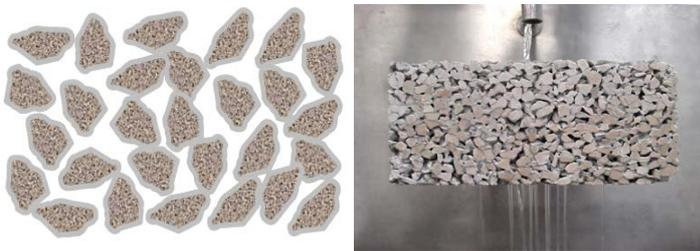
Figure 3: Pervious concrete conception
