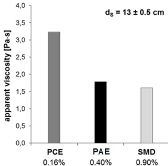
Figure 7: Apparent viscosity at constant slump flow
