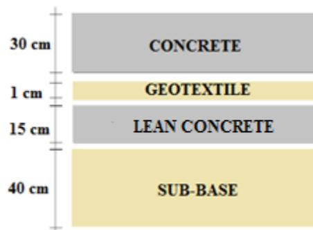
Figure 2: Section of the pavement
