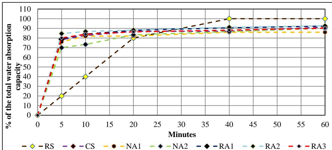
Figure 2: Aggregate water absorption over time, in percentage of the total absorption capacity
