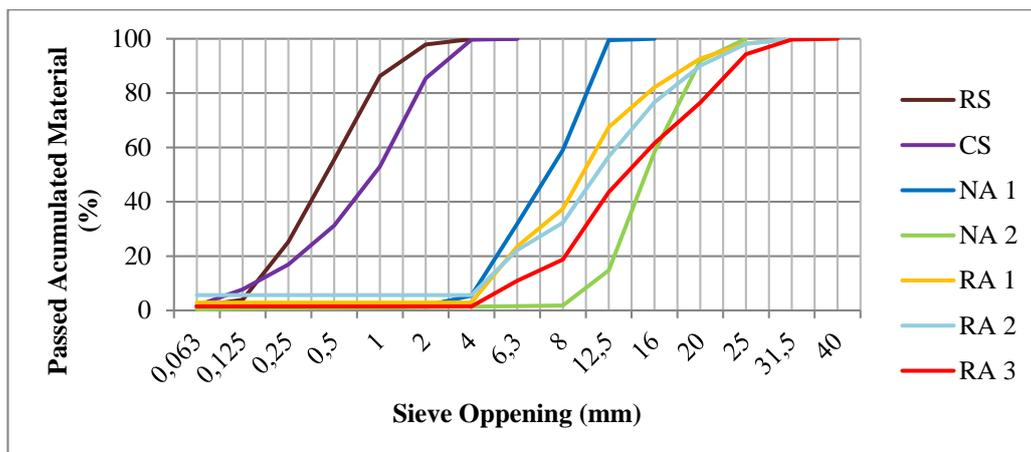
Figure 1: Aggregate sieve analysis
