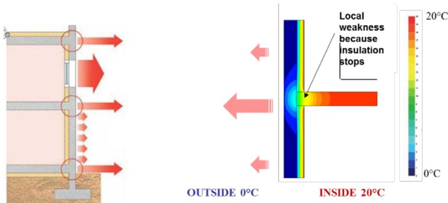
Figure 6: Thermal bridges
