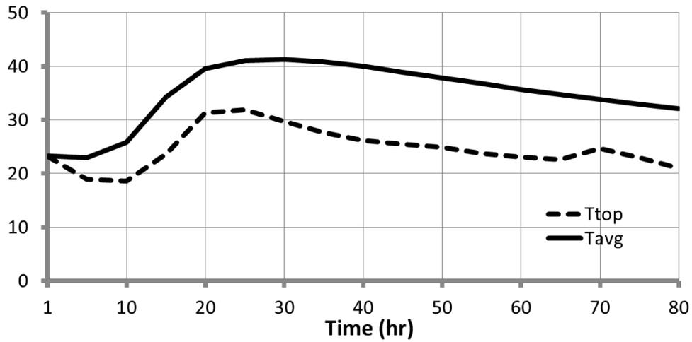
Figure 2: Typical average temperature-time and surface temperature-time curves for the first layer of the foundation.
