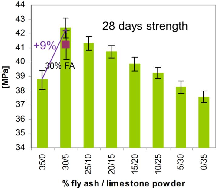
Figure 4: Comparing the 28 day compressive strength of composite cements with different combination of fly ash (FA) and limestone powder (L) from [11].
