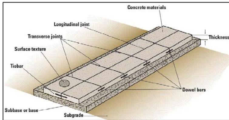
Figure 3: Joint Plain Concrete Pavement (JPCP)
