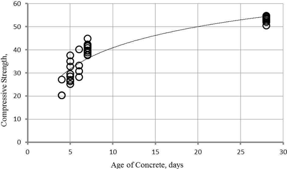
Figure 4: In cold weather conditions, relation between cylinder compressive strength and age of concrete for Mix 2
