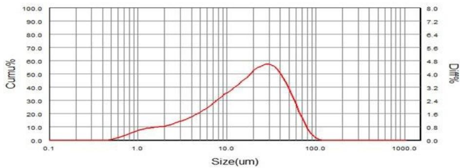
Figure 2: Particle size graphic of P-2 cement
