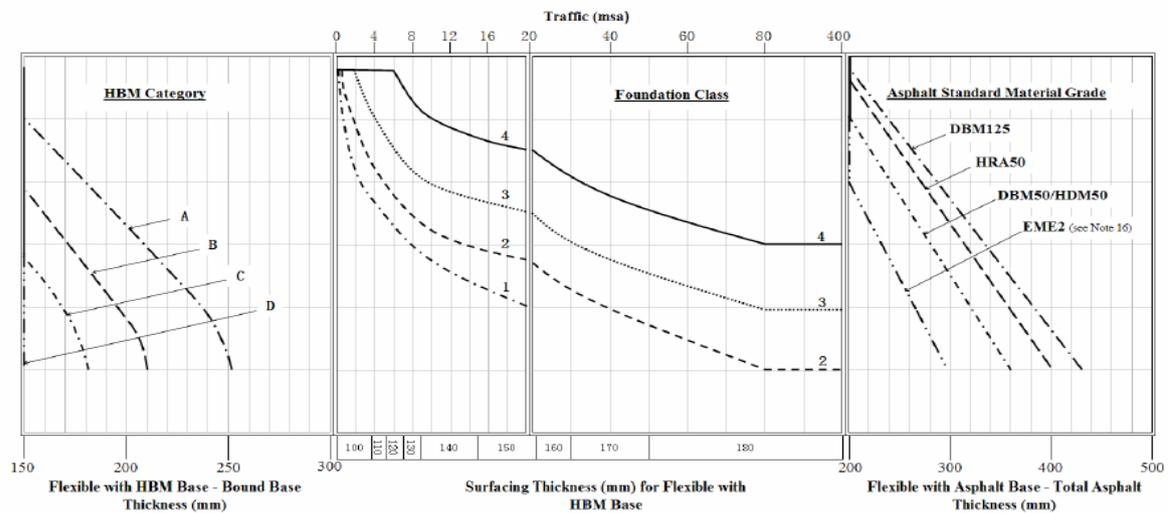
Figure 5: Design Chart for composite construction
