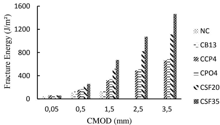
Figure 8: Fracture energy-CMOD of fiber reinforced and plain concretes.
