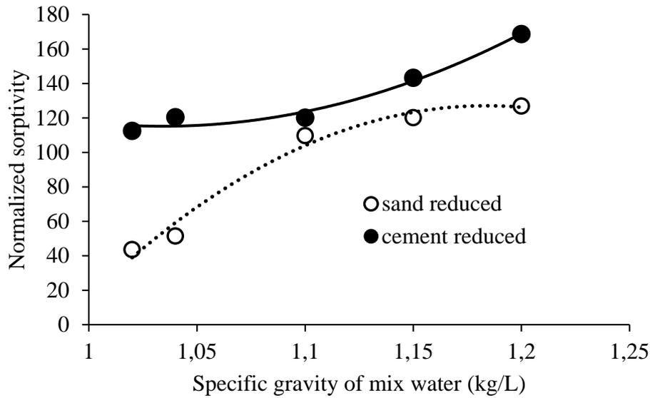
Figure 4: Normalized sorptivity of concretes at the age of 28 days
