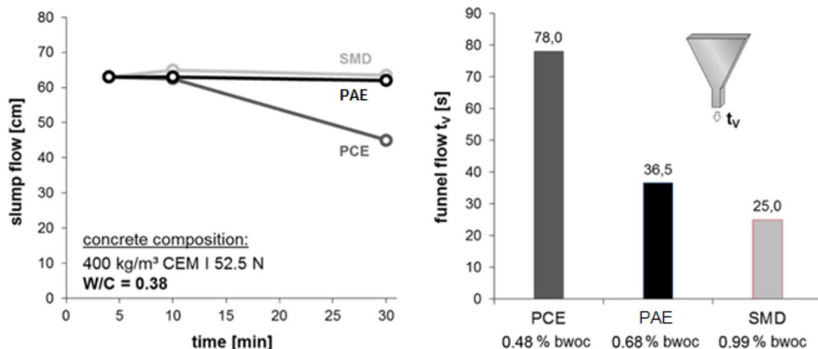
Figure 5: Slump flow behavior and V-funnel times for concrete prepared with PCE, PAE and SMD (concrete mixtures 1, 2, 3)
