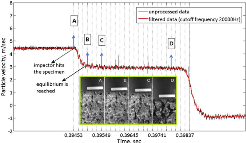
Figure 2: A representative particle velocity time history graph for the interface between the sample and the impactor used in impact stress calculations
