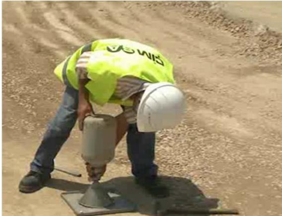
Picture 3: Sand cone test
