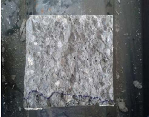
Figure 4: Marked depth of water ingress.
