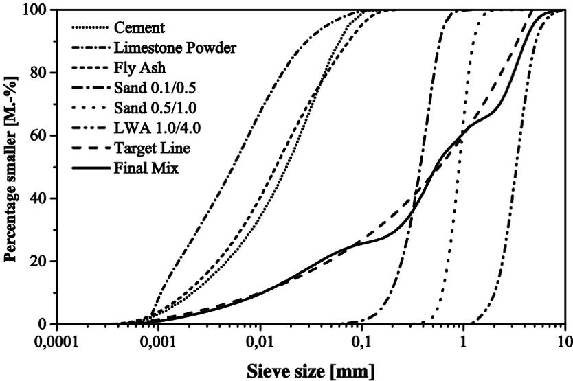
Figure 4: Grading of the materials used, target line and final mix
