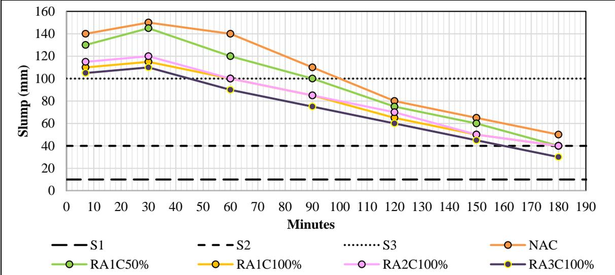
Figure 4: Slump test over time
