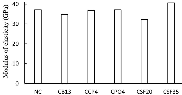
Figure 3: Elastic modulus of concrete mixes.
