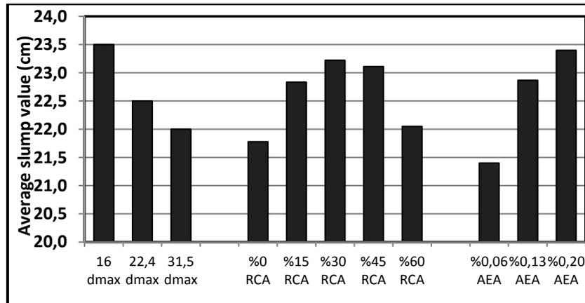
Figure 1. Average slump values by parameters
