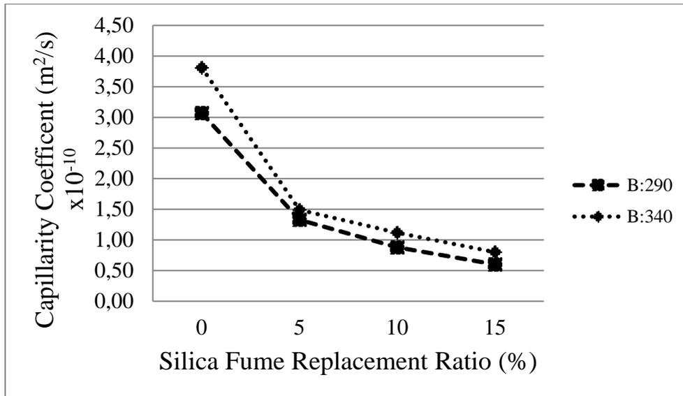
Figure 8: Capillarity coefficients measured on concretes.
