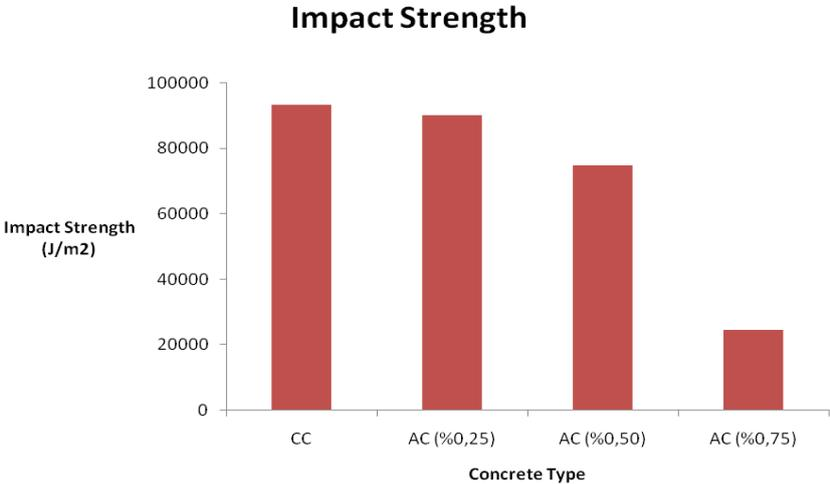
Figure 5. Graphical display of the results of the impact test
