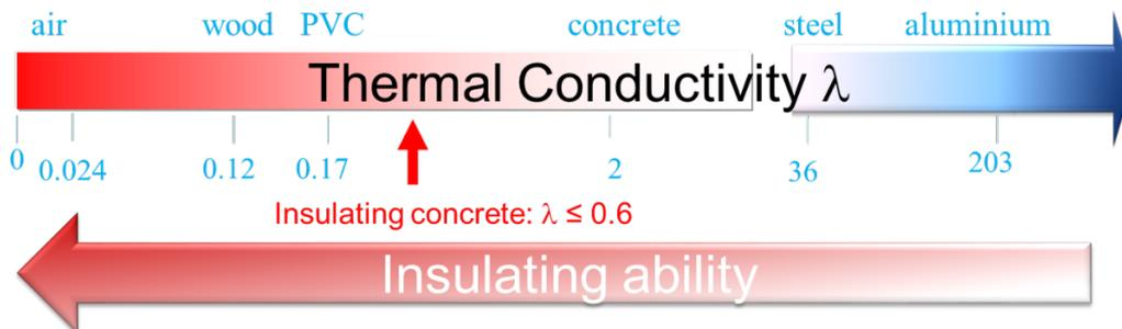
Figure 5: Thermal conductivity of materials
