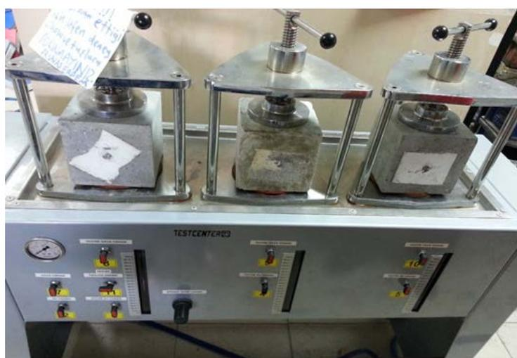
Figure 3: Water permeability testing apparatus
