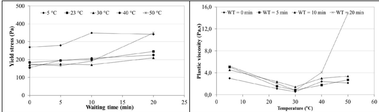
Figure 1: Variation of rheological parameters (a) Yield stress, (b) Plastic viscosity
