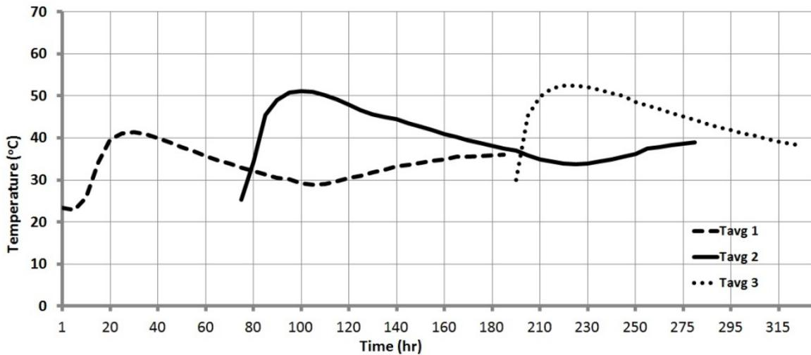
Figure 3: The average temperature versus time curves for the first, second and third layers.
