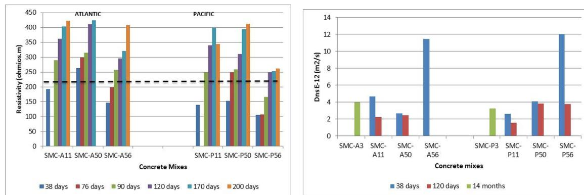
Figure 4: LEFT- Resistivity values up to 200 days and RIGHT- Diffusion coefficients at 38- and 120-day for all mixes except A3 and P3 (tested after 14 months only).
