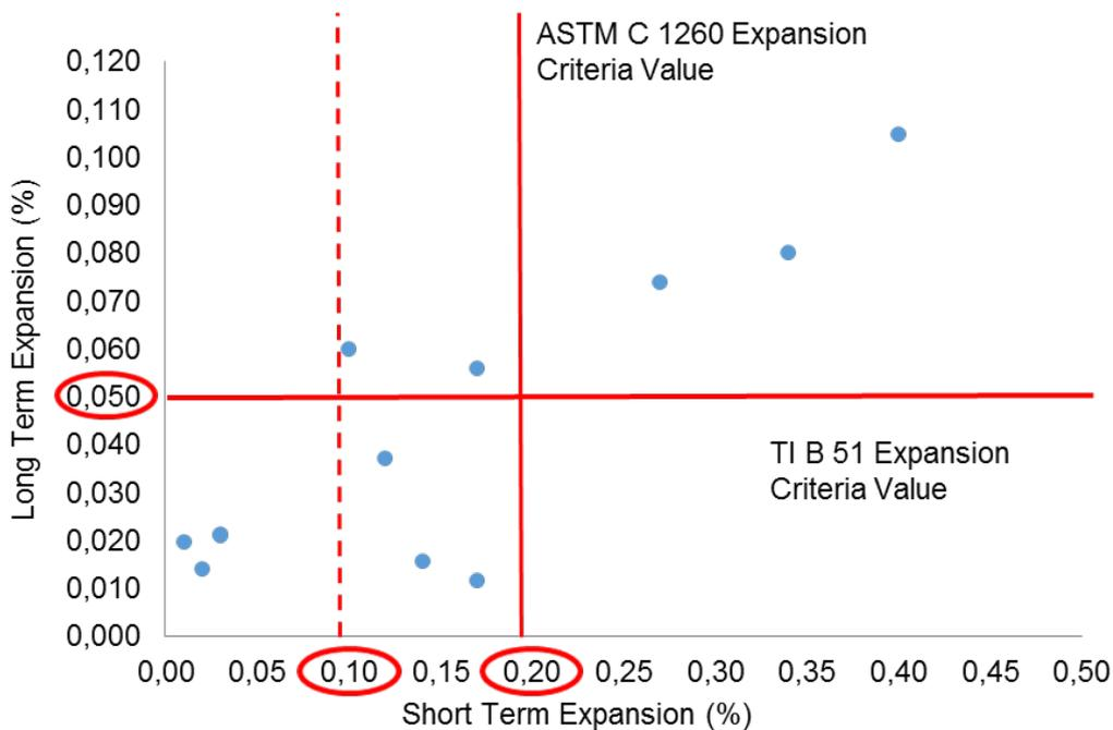
Figure 4: Short term and long term test results of 12 different mortar mixes
