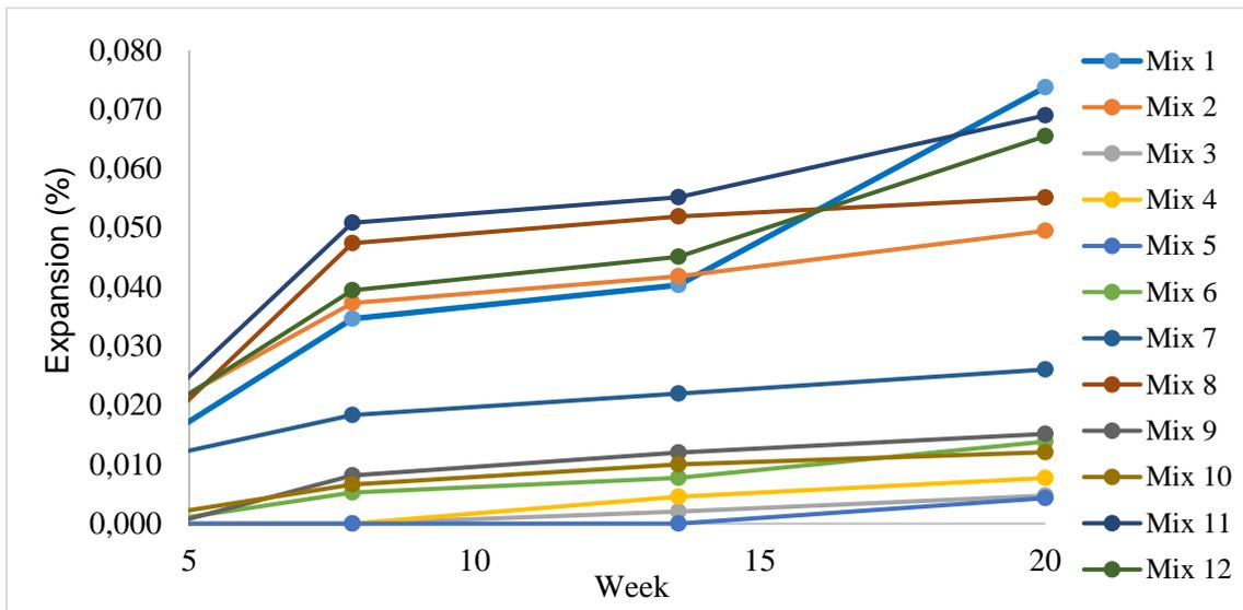
Figure 3: TI B 51 Test results of 12 different mortar mixes
