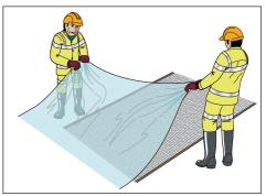
Figure 15. Polythene sheeting used to protect concrete.
