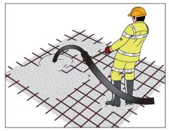
Figure 4. Placing concrete using a pump
