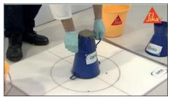
Figure B.11 Slump-flow cone ready for lifting
