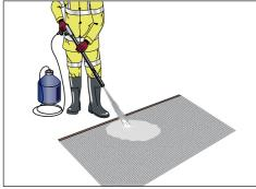
Figure 16. Spraying on curing membrane.
