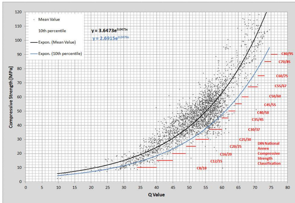
Figure 3: Relationship between cube strength and rebound number (Type Q)
