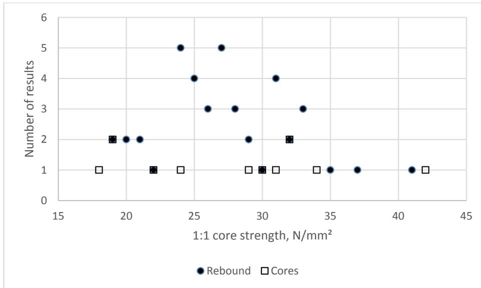
Figure 1: Distribution of strength in an element under investigation
