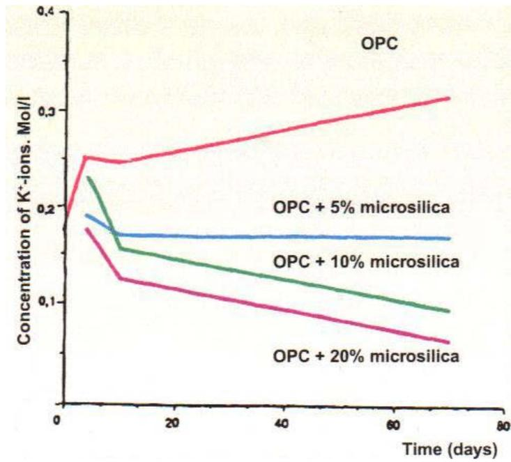
Figure 1: Reduction in Alkali ions with the addition of silica fume [1]
