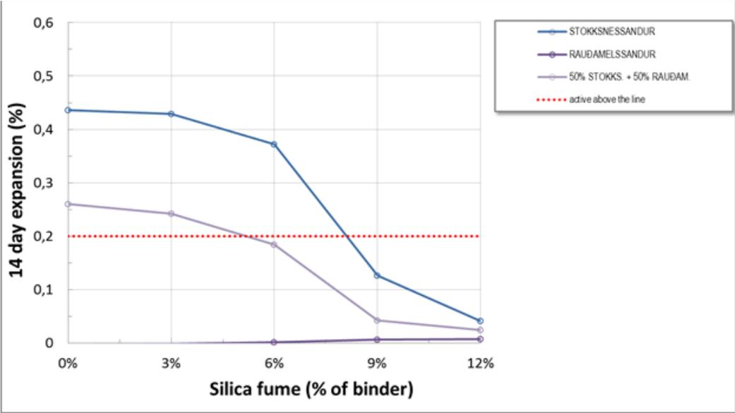
Figure 4: Expansion of individual and blended sand mixes with increasing silica fume [4]
