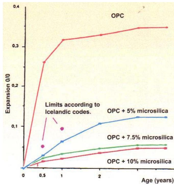
Figure 2: Reduction in Expansion with the addition of silica fume [2]
